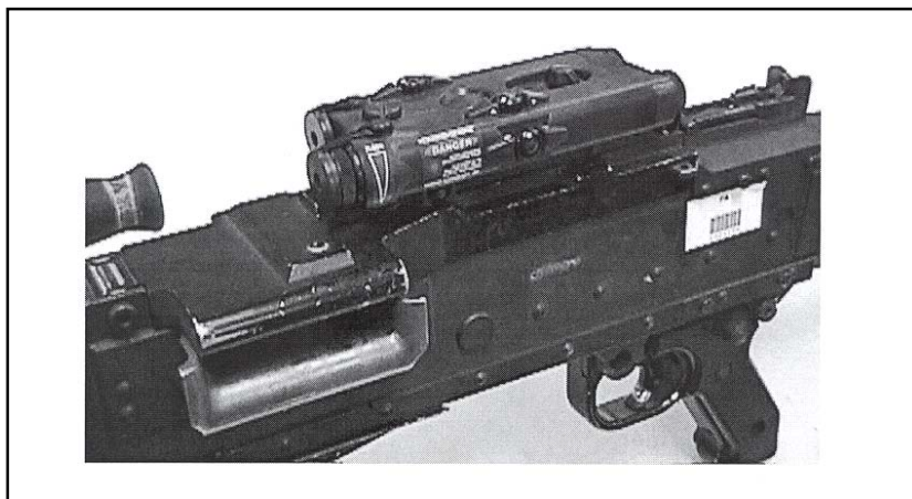
Figure G-20. Mounting the AN/PEQ-2A to the M240B machine gun.
