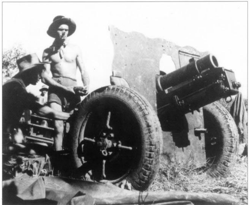
3.7in. howitzer in action in Burma. This howitzer was originally developed for the Indian Mountain Artillery. It was particularly useful in the jungle as it could be quickly dismantled for transport by mule or by manpower. (courtesy of the Trustees of the Imperial War Museum)
