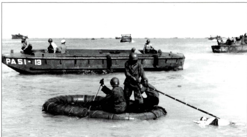
The APDs carried only four of the original unarmed Higgins boats, the Landing Craft, Personnel (LCP), to tow rafts toward shore or to use as platforms to make boarding the rafts easier in a high sea. They could not carry the heavier and more familiar Landing Craft, Vehicle, Personnel (LCVP). (National Archives)
