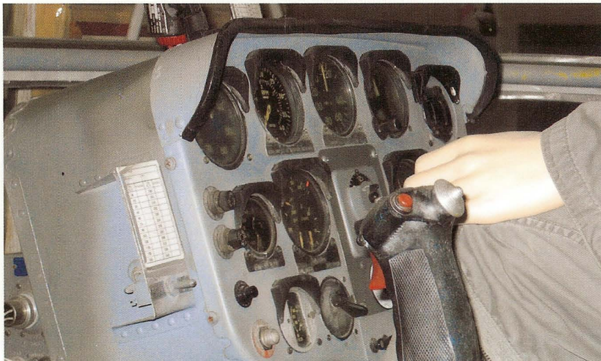
The simple instrument panel of the OH-13G was ideal for primary flight training. It was not so complex as to confuse the student.
