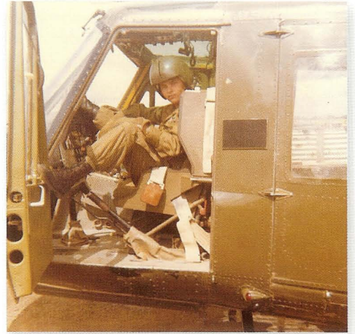
A UH-1H crew chief relaxes in a pilot's seat awaiting the order to launch a mission. Below his left leg is an angled black bar. This is the collective that controls blade pitch, and is also the throttle. (Kenneth Upton)
