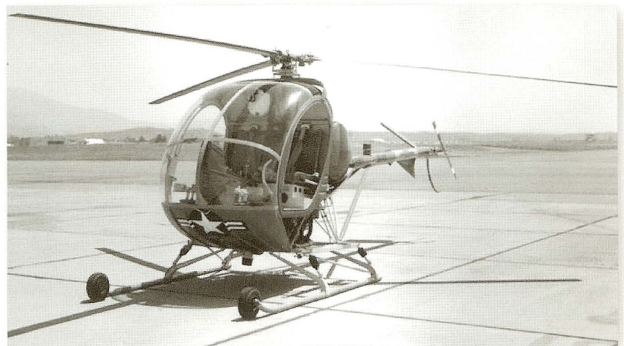
The OH-13G and OH-23D began to be phased out by the Hughes TH-55A Osage trainer. The earlier trainers were no longer in production and existing choppers were wearing out. The Osage was developed as a low-cost replacement.
