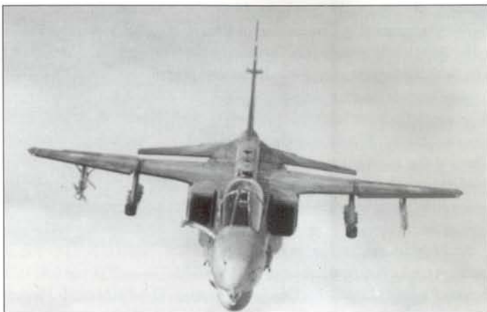
A French Armée de l'Air SEPECAT Jaguar A on close air support patrol over Bosnia armed with free-flight rocket pods (Tim Ripley)
