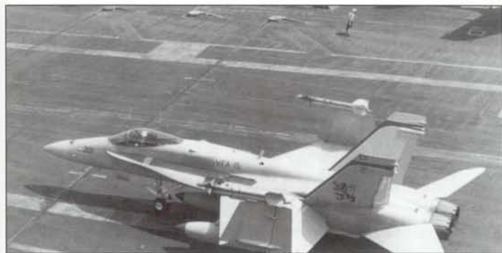
AGM-88 HARM armed McDonnell Douglas F/A-18C Hornets flew constant patrols to respond to SAM threats against allied aircraft operating over Bosnia (Tim Ripley)
