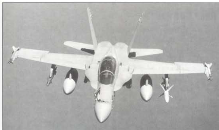
Two-seat USMC McDonnell Douglas F/A-18D Hornets, of VMFA(AW)-533 brought a true multi-role capability to NATO operations during 1995, flying with AIM-9 Sidewinder air-to-air missiles, Paveway laser guided bombs and AGM-88 HARM anti-radar weapons (Tim Ripley)
