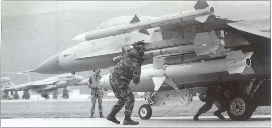
USAF ground crew pre-flight a Lockheed Martin F-16CJ Fighting Falcon armed with a AGM-88 HARM anti-radar weapons, AIM-120 AMRAAM and AIM-9 Sidewinder missiles (US DoD/JCC(D))
