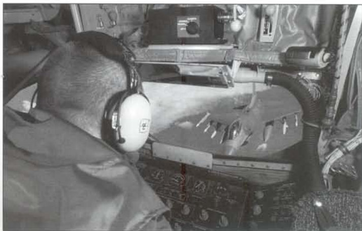
A boom operator of a Boeing KC-135R Stratotanker prepares to pass fuel to a fighter in a refuelling 'track' over Bosnia (US DoD/JCC(D))
