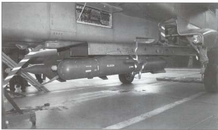
Royal Air Force Panavia Tornado strike aircraft equipped with TIALD designator pods carried out daily raids on Yugoslavia (RAF)
