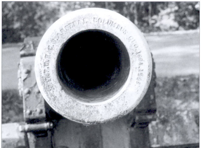
The muzzle of a Napoleon made by the Columbus, Georgia, Arsenal bearing, clockwise from left, the inspector's initials, "C.S ARSENAL COLUMBUS GEO. 1864," and the weight of the tube. (Gettysburg National Battlefield Park)
