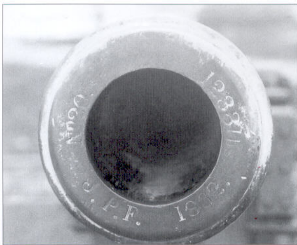
The markings on the muzzle of the M1857 12-pdr. include, clockwise from left, the weapon number, the weight of the tube, the date of manufacture, and the inspector's initials.
