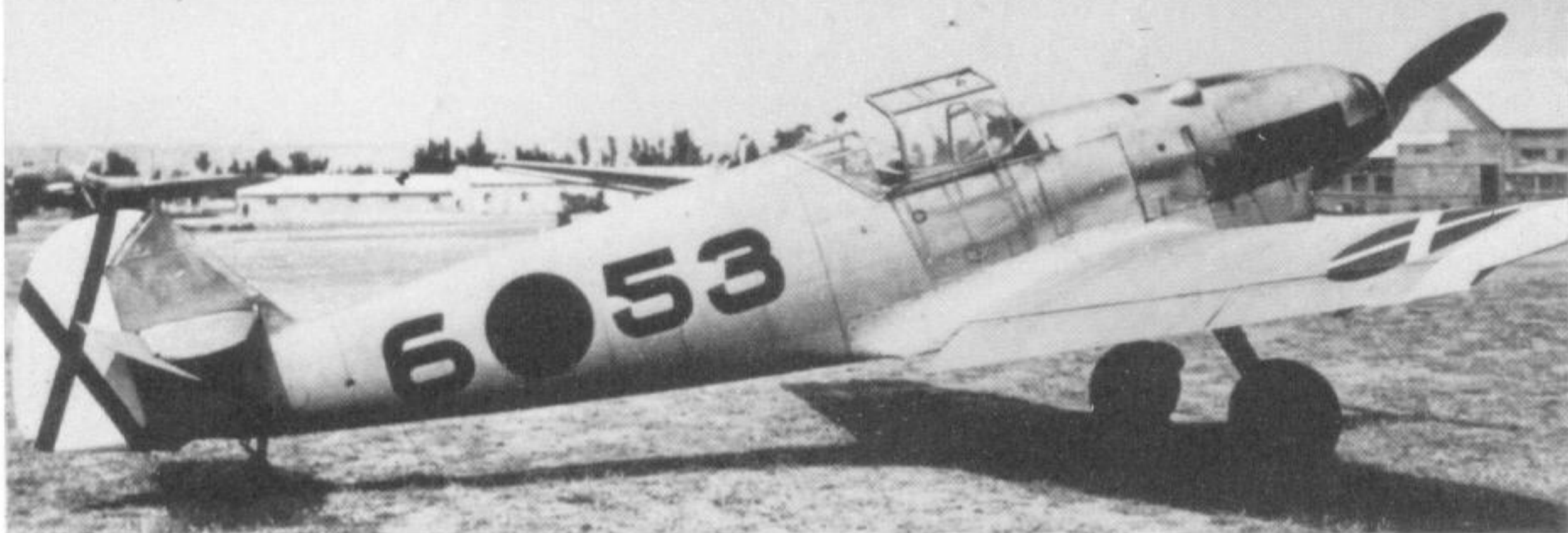
✓ Above: Messerschmitt Bf 109B-2 2./J88 Legion Condor, Brunete area, near Madrid, Spain, June 1937. At the time the photograph was taken the "Top Hat" insignia had not been applied to the fuselage; note the wing roundels slightly overlap the ailerons. (Hans Obert)
