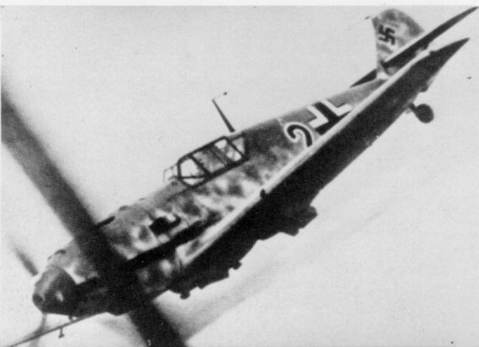
Bf 109E-7/U2; this version was very heavily armoured for ground-attack missions and used extensively in the desert campaigns. (F. Selinger via M. C. Windrow)
