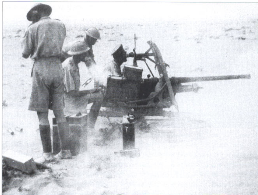
The British 2-pdr Mk I AT gun weighed 1,858lb, about twice as much as its US and German 37mm counterparts. It could be fired from its wheels, but they were normally removed for action and the gun set up on its integral three-legged mounting. Side shields were available, but seldom used.
