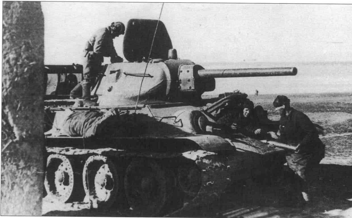
A Soviet T-34 Model 41/42 tank prepares for battle. The crew is loading shells through the driver's hatch. (Paul McDaniel)
