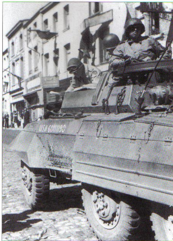
The M20 armored utility car was widely used by senior commanders in the summer and fall of 1944 before its vices became evident. This is the vehicle of Maj. Gen. "Lightning Joe" Collins, commander of the VII Corps which led the Normandy breakout during Operation Cobra. Here, he is checking his map in the Belgian town of Beaumont on September 4 1944. (NARA)
