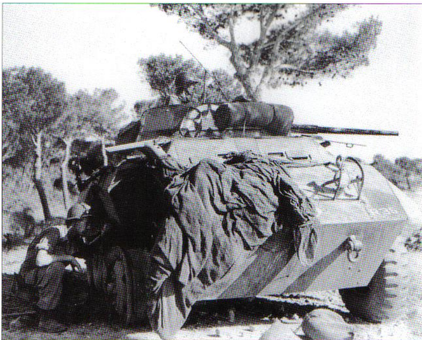
One of the main problems with the M8 armored car in Italy was its vulnerability to mines. The floor had no armor, which led to high crew casualties when mines were encountered. One of the crewmen of this M8 looks over the damage while the turret crew keeps watch near Castiglione on July 13 1944. This particular vehicle served with a tank destroyer reconnaissance company. (NARA)
