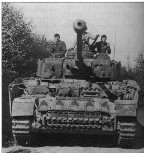
The final production version of the PzKpfw IV, the Ausf. J, dispensed with the power traverse system in favour of an increased fuel capacity. The crew of this vehicle have made good use of captured T-34 and other track links. (Bundesarchiv)
