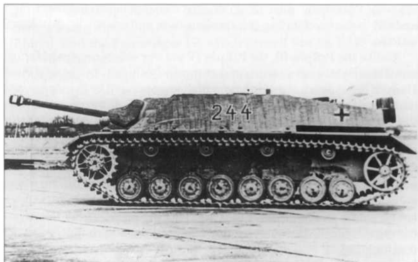
The Panzerjäger IV was a second-generation tank destroyer mounting first an L/48 (as seen here) and later an L/70 75mm gun. The vehicle displays a full coating of zimmerit anti-magnetic mine paste.
