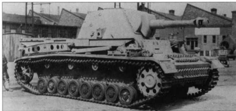
The Heuschrecke (Grasshopper) was armed with the light 105mm howitzer, and was based on a slightly lengthened version of the standard PzKpfw IV chassis. (RAC Tank Museum)
