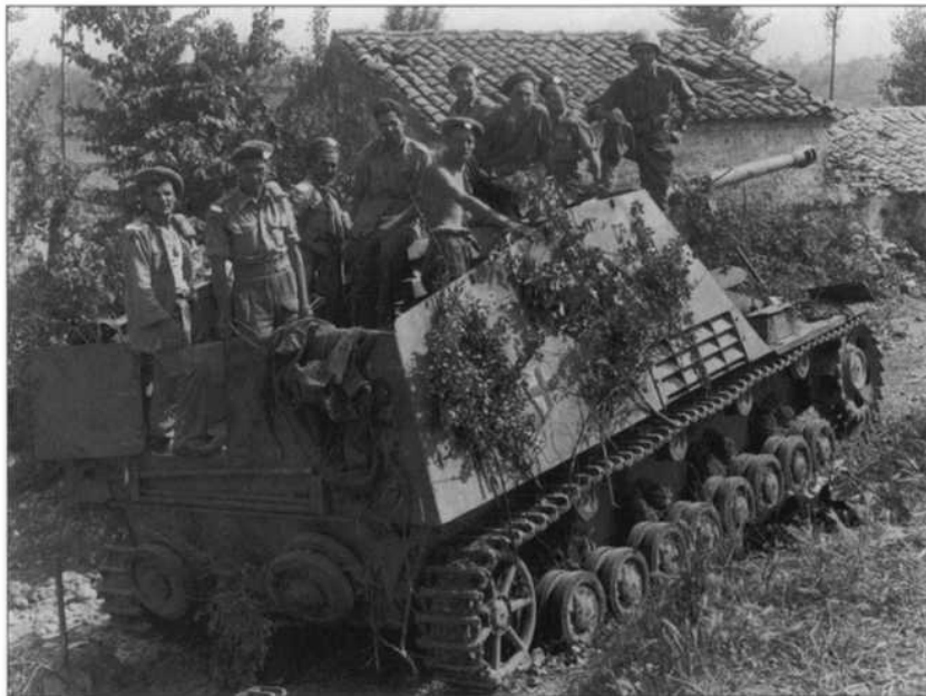
The Nashorn (Rhino) was a first-generation heavy tank destroyer and was armed with the L/71 PAK 43/1 88mm anti-tank gun. This example was stalked and killed with a PIAT by Canadian infantry near Pontecorvo, Italy. Unfortunately, the censor has erased every detail of cap badges and shoulder titles. (Public Archives of Canada)
