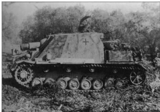
The massive construction of some buildings encountered during the street fighting in Stalingrad induced a demand for a heavy assault gun. The result was the Brumbär (Grizzly Bear), based on the PzKpff chassis, which mounted a 150mm L/12 howitzer in a fixed superstructure. (US National Archives)
