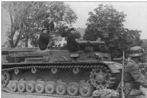
This Ausf. B probably belonged to the same unit and is identifiable by the straight front plate incorporating the hull machine-gun. The vehicle carries a small fascine for unditching purposes. See Plate A1. (Bundesarchiv)
