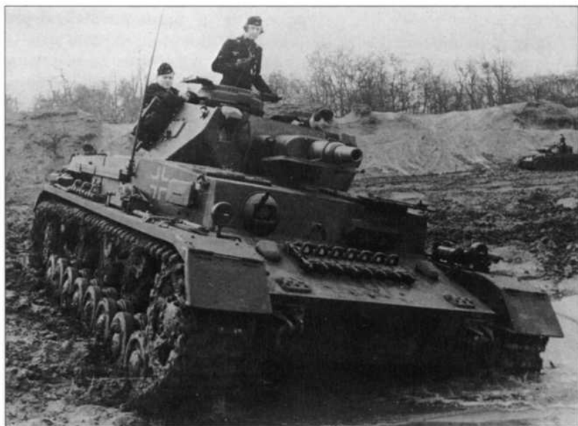
The Ausf. F1 carried 50mm frontal armour and had wider tracks than previous marks. Note the deflector rail under the gun, designed to push back the aerial when the turret was traversed to the right. (Bundesarchiv)
