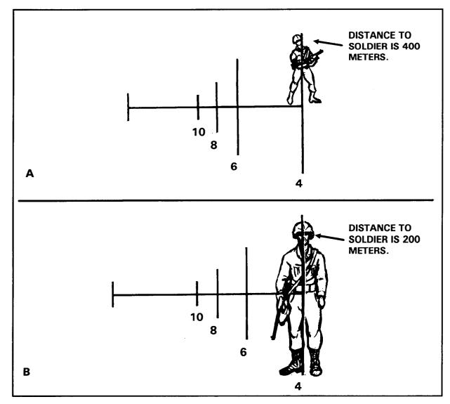
Figure 6-5. Range estimation using the AN/PVS-4 nightsight.
