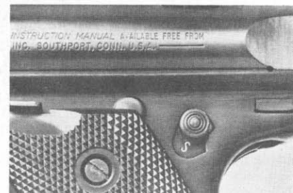
Figure 2. Safety in the "on" or "safe" (S) position. Safety is all the way up .
