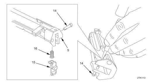
7. Place 1/8 in. punch on split end of sear pin (14) and lightly tap punch with hammer to dislodge pin. Remove sear assembly (15) and sear spring (16) from bolt carrier (5).
