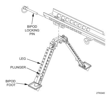
1. Grasp lower receiver. Extend bipod legs by pulling legs down to front, where they will lock into place. Pulling on feet of bipod causes legs to extend. To retract a leg, depress plunger located on bipod leg and push on foot. Place receiver on level surface. Pull down on leg and wing back into position along receiver.
