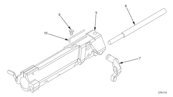
3. Remove accelerator (7) by pulling it from left side of bolt carrier (5). If necessary, a punch may be used to assist with removal. Slide accelerator rod (8) from rear of bolt carrier.
