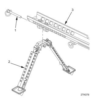
Remove bipod locking pin (1) by pulling on ring to separate bipod assembly (2) from lower receiver assembly (3).
