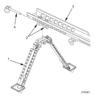
Align bipod assembly (1) with yoke mounts (2) on lower receiver assembly (3) and secure with bipod locking pin (4).
