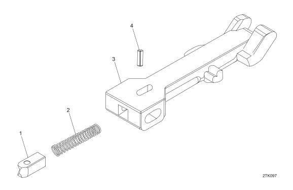
Figure 3. Transfer Bar Assembly, 82074-1A.
