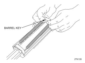
e. Slide barrel back into receiver and rotate 1/2 turn.
