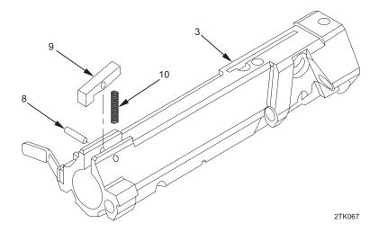
4. Use 1/8 in. pin punch and hammer to tap out bolt latch pin (8). Remove bolt latch (9) and bolt latch spring (10) from bolt carrier (3).
