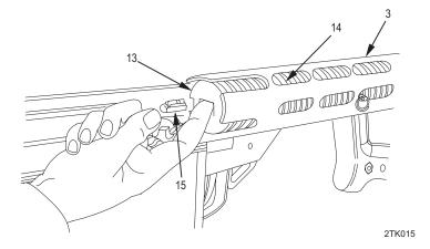
6. Place fingertip into slot on mainspring buffer (13), and turn buffer so that groove in its flange lines up with buffer stop (15) on lower receiver (3). Slowly and carefully remove mainspring buffer and mainspring (14).
