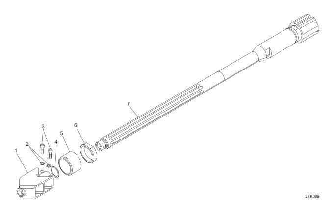
Figure 9. Barrel Assembly, DBC-005.
