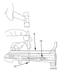
8. Compress cam pin spring against bolt carrier (9) until cam pin assembly (12) slips into its groove. While holding down cam pin assembly, insert spring pin (13).
