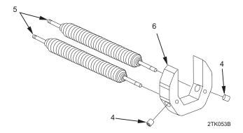
3. Use 1/8 in. hexagon wrench to remove barrel spring screws (4). Remove two barrel springs (5) from barrel key (6).
