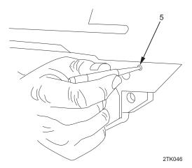
2. Remove transfer bar pin (5) (behind safety in trigger housing) by placing 5/32 in. punch on pin and tapping it out with hammer.
