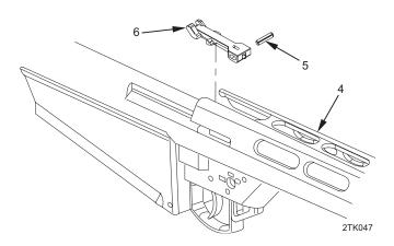
3. Remove transfer bar assembly (6) from lower receiver (4).
