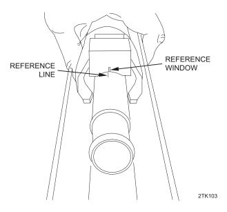
b. If the reference line on the test bolt falls within the reference window, then a #10 bolt is required.
