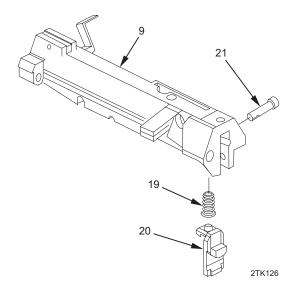
12. Insert sear spring (19) and sear assembly (20) into bolt carrier (9). Insert split end of sear pin (21) into charging handle side of bolt carrier and tap in with hammer.
