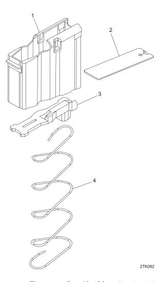
Figure 14. Cartridge Magazine, 82116A.
