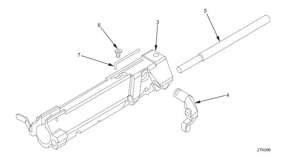
2. Remove accelerator (4) by pulling it from left side of bolt carrier (3). If necessary, a pin punch may be used to assist with its removal. Slide accelerator rod (5) from rear of bolt carrier.
