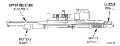
2. Carefully pick up upper receiver assembly. Barrel will be nested inside it for compact storage. Move bumper rings into position on either side of receiver's central barrel bushing, so that they rest snugly against bushing. Align barrel so that its feed ramp (slanted entry to firing chamber) is to bottom. Keeping fingers away from barrel, hold upper receiver horizontally and then tilt in direction of muzzle. Barrel should fall into place, at its full forward extension in receiver.
