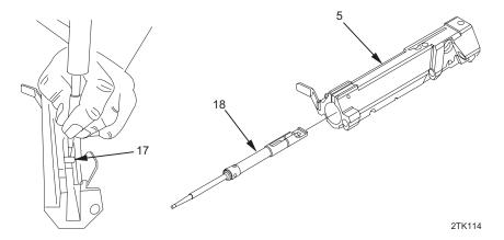
8. Place 1/8 in. punch on split end of extension stop pin (17) located on underside of bolt carrier (5). Lightly tap punch with hammer to dislodge pin and remove firing pin extension assembly (18) from bolt carrier (5).
