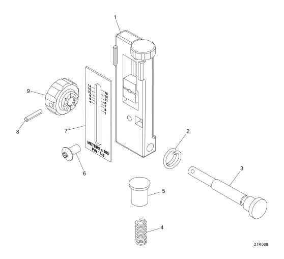
Figure 8. Iron Sight Assembly, 8SA2.
