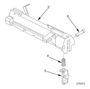
3. Insert sear spring (4) (tapered end first) and sear (5) into bolt carrier (2). Insert split end of sear pin (6) into bolt handle side of bolt carrier and tap in with brass hammer.
