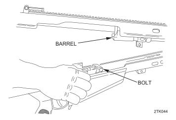
5. Lower and close upper receiver onto lower receiver. Release charging handle slowly until bolt engages barrel.
