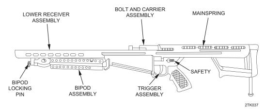
a. The bolt and carrier assembly is held in place under tension in the lower receiver by the midlock pin, which extends through a locking hole in the receiver's sheet metal.
