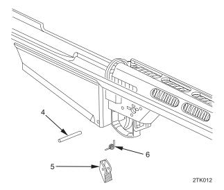
Place 1/8 in. pin punch on magazine catch pin (4) and tap pin out with hammer. Remove magazine catch (5) and magazine catch spring (6).
