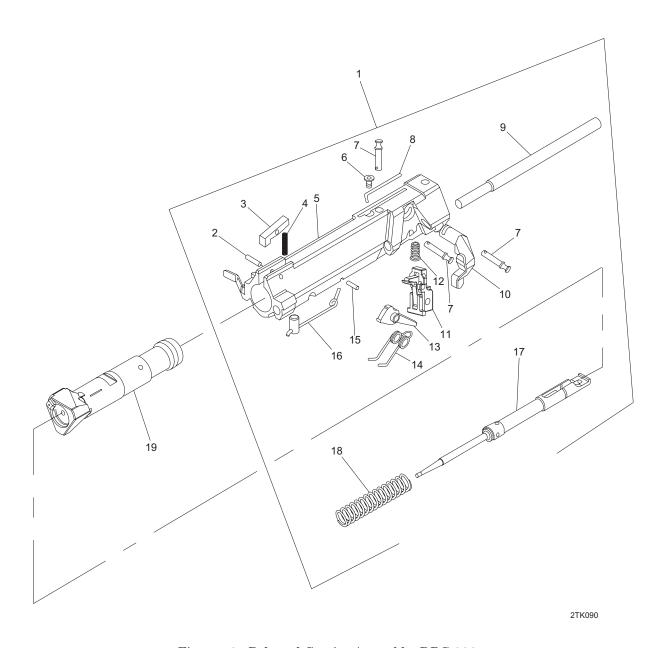
Figure 10. Bolt and Carrier Assembly, DBC-006.
