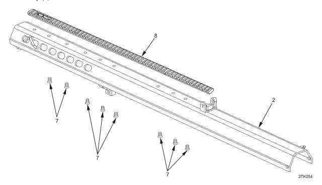
4. Remove eight scope base screws (7) and scope base (8) from upper receiver (2). Remove old thread-locking compound from threads of screws.
