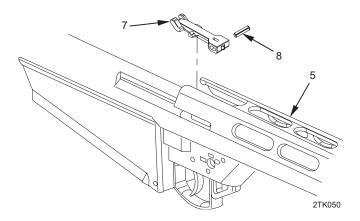
7. Place transfer bar assembly (7) into lower receiver (5). Install transfer bar pin (8) to secure transfer bar assembly.
