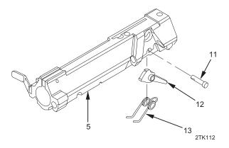
6. Remove cocking lever pin (11), cocking lever (12), and cocking lever spring (13) from bolt carrier (5).
