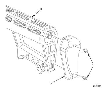
1. Using 5/32 in. (T-27) Torx screw key, loosen and remove two recoil pad screws (1). Remove recoil pad (2) from lower receiver (3).
