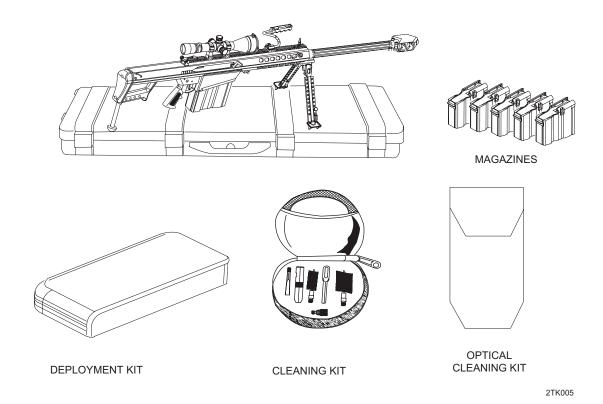
The M107 Rifle System comprises the rifle with a fixed variable 4.5X14 power sniper scope, and 6 magazines. The rifle is also supplied with a fitted dirt-tight and watertight carrying case, cleaning kit, and telescope adjustment tools.
