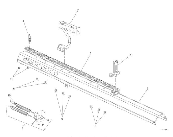
Figure 5. Upper Receiver Assembly, DBC-004.
