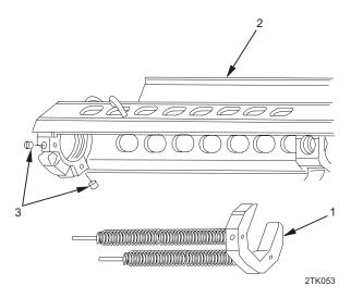
2. Use 1/8 in. hexagon wrench to remove two barrel spring screws (3) from front barrel bushing of upper receiver (2). Drive springs of barrel key assembly (1) from front of upper receiver with 3/32 in. punch. Remove old thread-locking compound from barrel spring screws.
