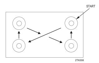
b. Tighten scope ring screws (1) evenly and securely. Start in one corner and tighten a small amount; then tighten the screw in the opposite corner. Tighten the screw above/below and then across corner. Continue the pattern until all screws are tightened; this ensures an even tightening and prevents skewing of the scope.
