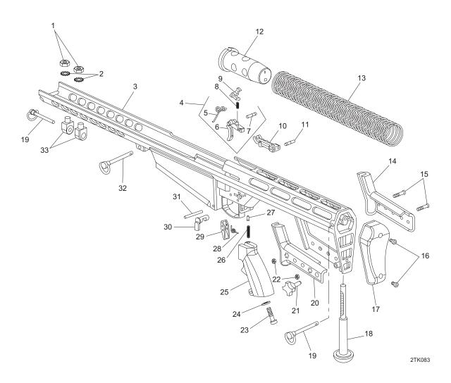
Figure 2. Lower Receiver Assembly, DBC-002, and Trigger Assembly, 82069-2A.
