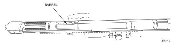
f. Retract bolt until hole in bolt is visible through first hole in lower receiver. Insert midlock pin into hole.
