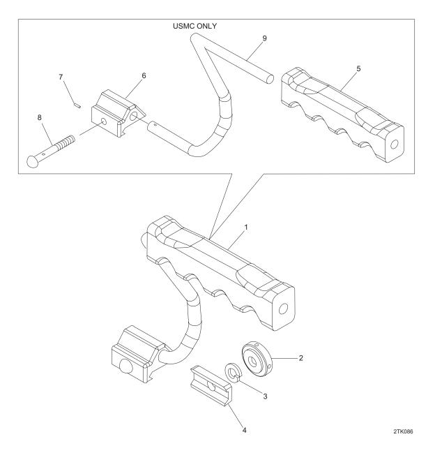
Figure 6. Carrying Handle Assembly, 82048-C3.
