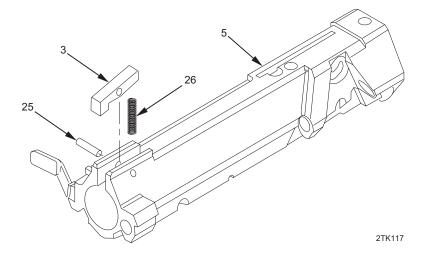
12. Use a 3/32 in. punch and hammer to tap out headless straight pin (25). Remove bolt latch (3) and compression helical spring (26) from bolt carrier (5).
