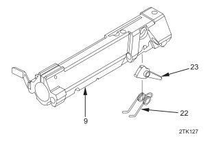
13. Place cocking lever spring (22) on cocking lever (23). Insert both into underside of bolt carrier (9) with ends of spring pointing forward on either side of firing pin.
