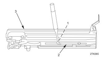
1. Place 1/16 in. pin punch on cam pin (1) and tap punch lightly with hammer. Remove cam pin and cam pin assembly (2) from bolt carrier (3).
