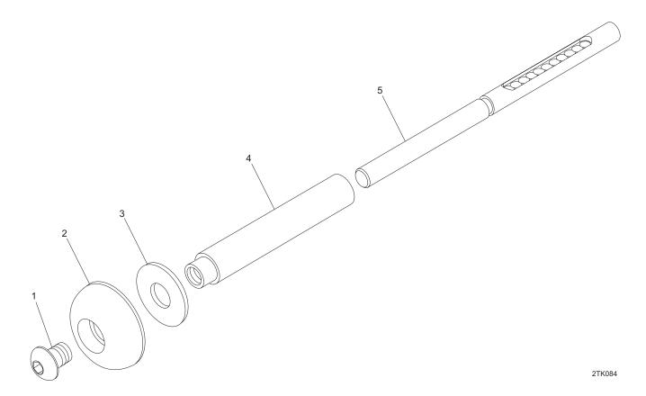
Figure 4. Monopod Assembly, 82226-A.
