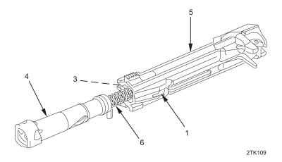
2. While holding up cam pin assembly (1), depress bolt latch (3) on its rearward portion. Bolt assembly (4) should spring forward. Grasp bolt assembly and remove from bolt carrier (5). Use care not to lose or deform bolt spring (6).
