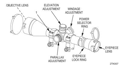
a. There are seven basic parts to the daylight scope: the objective lens (front lens), the elevation adjustment turret, the windage adjustment turret, the power selector ring, the eyepiece lock ring, the eyepiece lens, and the parallax adjustment turret (left side).
