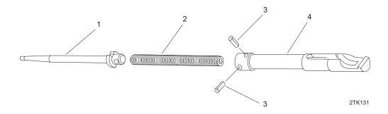
Figure 13. Firing Pin Extension Assembly, 82097-1A.
