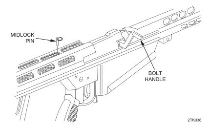
Standing above and to the rear of the lower receiver, grasp the bolt handle with the right hand and carefully pull back, against tension, while withdrawing the midlock pin from its retaining hole. Allow the bolt carrier to come forward SLOWLY until there is no more spring tension and it rests in the lower receiver.
