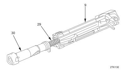
17. Install bolt spring (29) and bolt assembly (30) into bolt carrier (9), with cam groove to bottom.
