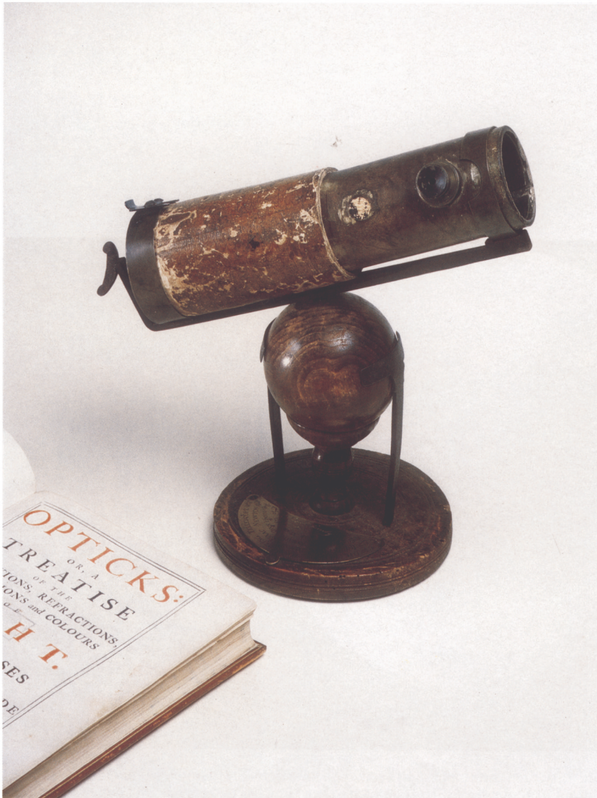
Plate 4 The first reflecting telescope, designed and built by Isaac Newton, which still exists in the rooms of The Royal Society in London. Also shown is the title page of his treatise on Opticks . The light enters the tube on the right-hand side and strikes a concave mirror at the base, from which it is reflected upwards in a converging beam to strike a plane, inclined mirror which reflects it out sideways where it can be viewed by the eyepiece shown. All major modern telescopes are reflecting in nature but the flat, inclined mirror is replaced by a curved, convex mirror which reflects the light back down the tube and through a hole in the centre of the primary mirror where it can be viewed or processed.
