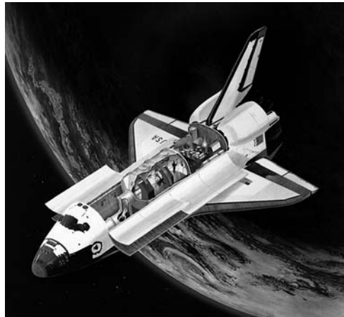
Artist's concept of the Spacelab-1 module and pallet in the Shuttle's payload bay.
