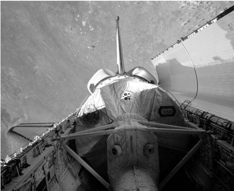
Orbiting in a gravity gradient attitude, Columbia’s port-side payload bay door is in a 62-degree-open position to protect its radiators from orbital debris impacts.
