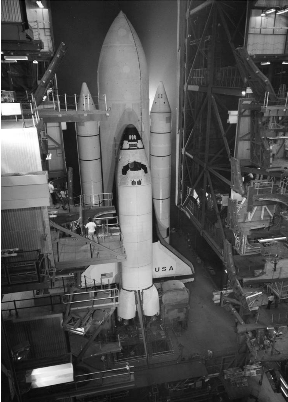
Attached to her External Tank and Solid Rocket Boosters, and mounted on top of the crawler, Columbia is readied for her first launch.
