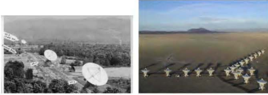
Figure 11.2. The Green Bank Interferometer (GBI; left) which was instrumental in detecting Sgr A* and the Very Large Array (VLA; right). Both interferometers are operated by the National Radio Astronomy Observatory (NRAO) in the United States and were extensively used to monitor the variability of Sgr A*.
