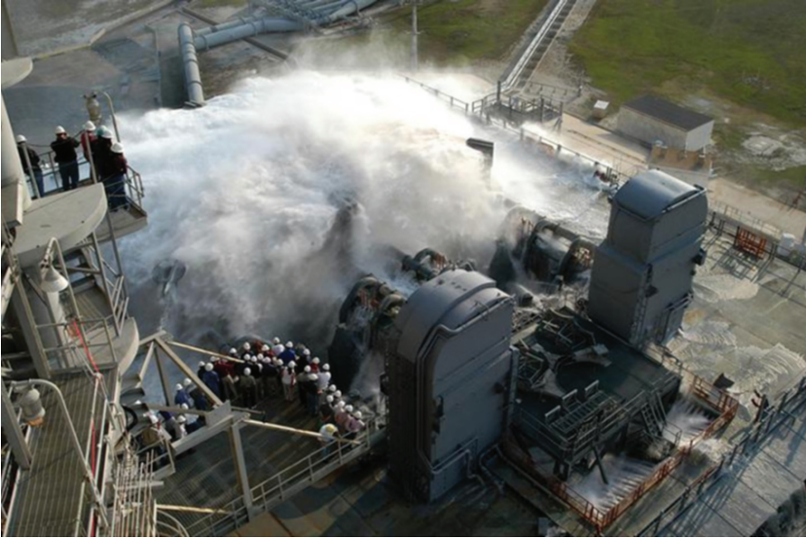
FIGURE 3.1 Sound Suppression Test. The Water Protects the Space Shuttle During Launch. Image courtesy NASA/KSC
