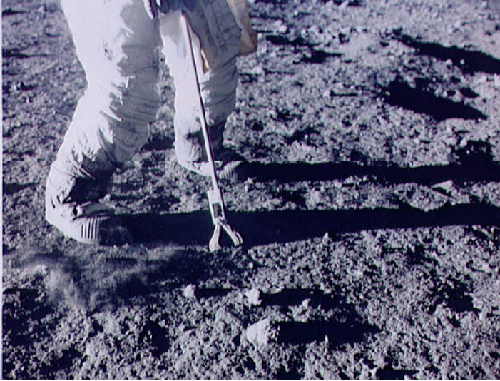
FIGURE 10.1 Close-up View of a Set of Tongs Being Used by Astronaut Charles Conrad Jr., to Pick Up Lunar Samples During the Apollo 12 Extravehicular Activity. Image courtesy NASA
