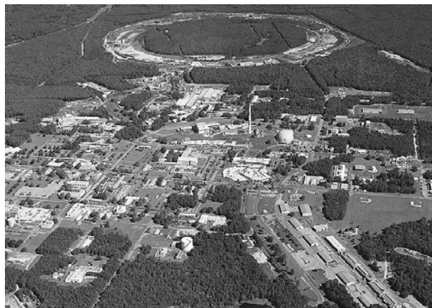
Brookhaven National Laboratory. The circle at the top is the Relativistic Heavy Ion Collider, which is 2.4 miles in circumference. CREDIT: COURTESY OF BROOKHAVEN NATIONAL LABORATORY. REPRODUCED BY PERMISSION.
