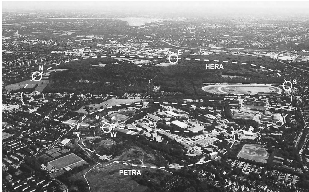
An aerial view shows the layout of PETRA (small ring) and HERA (large ring) at DESY in Germany. On Hera's North side (N) is the H1 detector, while ZEUS is located on the South side (S). HERMES is located on the East side (E). HERA-B is located on the West (W), closest to PETRA. CREDIT: COURTESY OF DEUTSCHES ELEKTRONEN-SYNCHROTRON (DESY). REPRODUCED BY PERMISSION.
