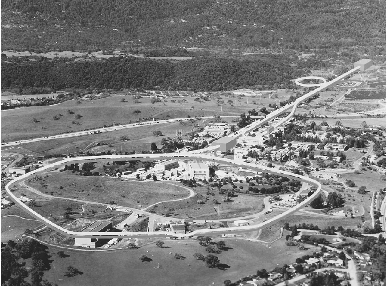
Aerial view of the Stanford Linear Accelerator Center (SLAC) with the linear accelerator (upper right) and PEP-II collider highlighted. Electrons from the electron gun and positrons from the positron source are accelerated in the linear accelerator. In PEP-II (large ring) the electrons and positrons circulate in opposite directions. These particles then collide in the BABAR detector, creating B mesons and anti-B mesons. Differences in these particles' rates of decay may help explain why there is more matter than antimatter in the Universe. CREDIT: COURTESY OF STANFORD LINEAR ACCELERATOR CENTER/SCIENCE PHOTO LIBRARY/PHOTO RESEARCHERS, INC. REPRODUCED BY PERMISSION.
