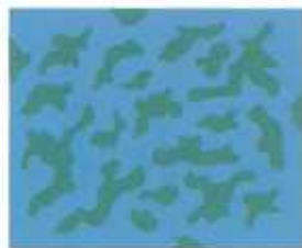
Fig. 17. Schematic drawing of the intermediate state of a superconducting plate. The magnetic field is normal to the plane of the paper.
