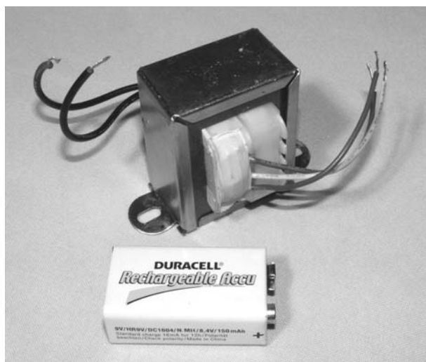
Figure 7-5 An AC transformer and a battery
