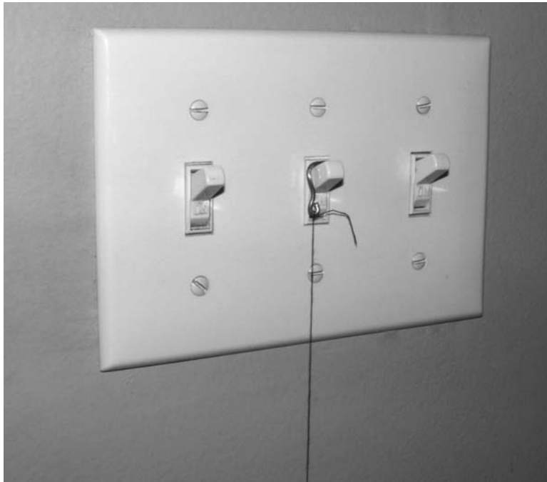
Figure 6-25 The servo can now pull the light switch off
