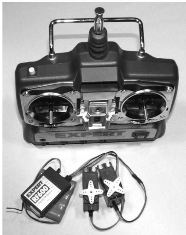
Figure 6-8 A typical hobby RC joystick and servo setup
