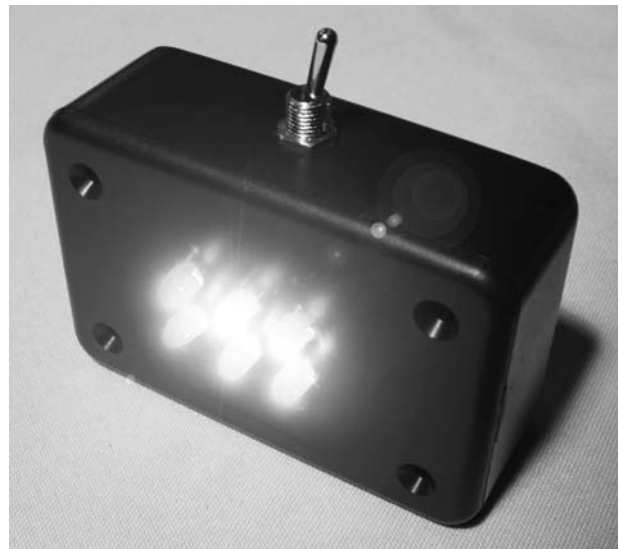
Figure 5-31 LED light projector completed
