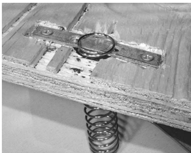
Figure 3-24 The spring is secured to the base
