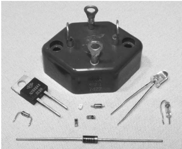
Figure 1-10 Several styles of diodes
