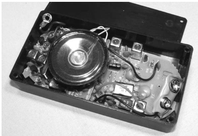
Figure 9-6 Re-fitting the receiver in a smaller box
