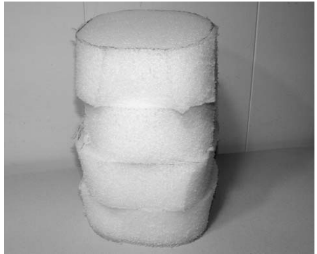
Figure 6-18 Foam disks glued and ready to cut
