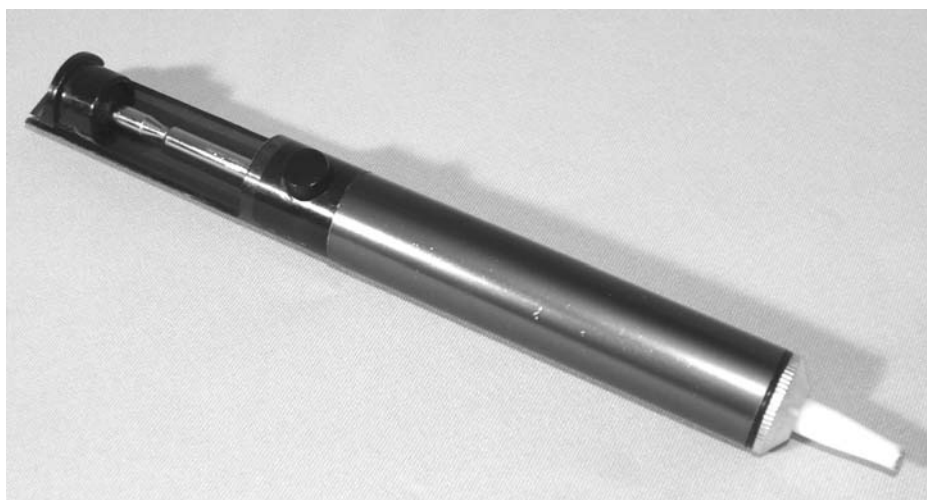
Figure 1-2 A solder sucker tool
