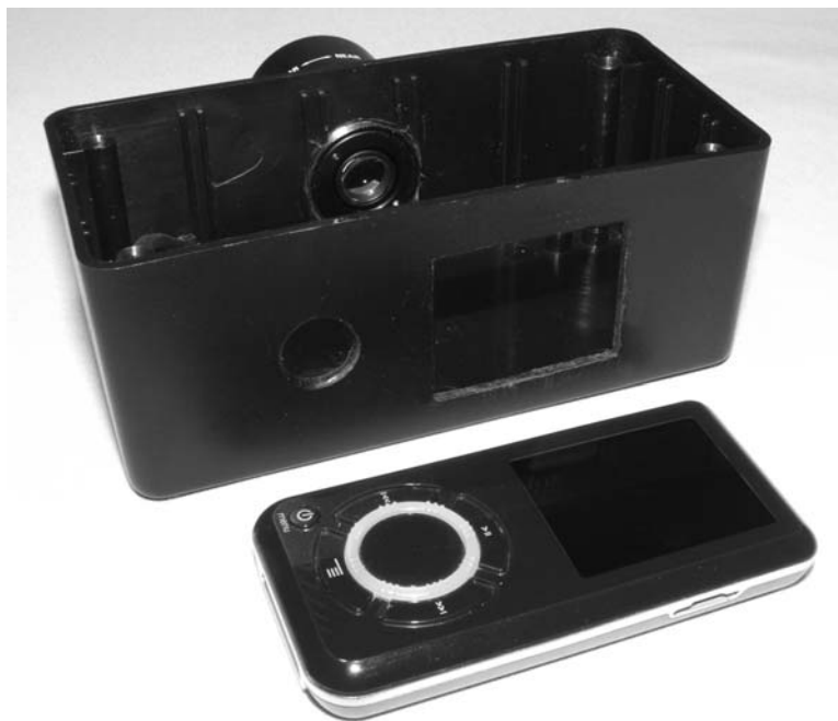
Figure 8-20 Enclosure holes cut for the video player
