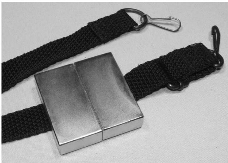
Figure 6-32 Installing the magnets to the leg belt
