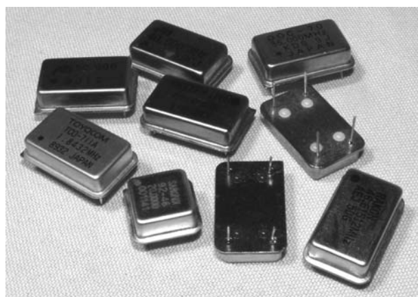
Figure 4-9 Several clock oscillators
