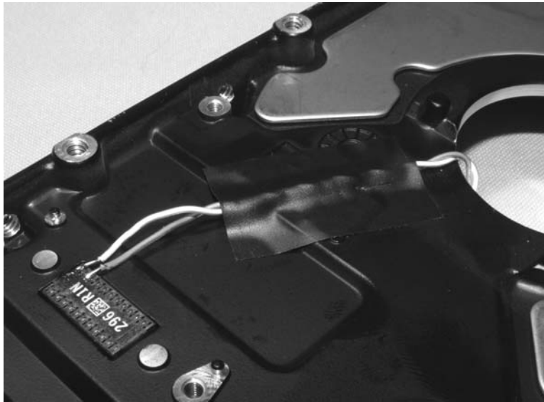
Figure 4-24 Voice coil electromagnet connection points
