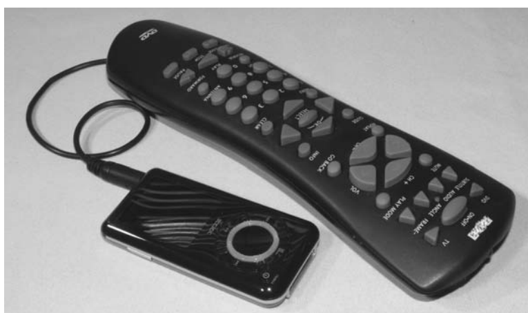
Figure 6-4 Audio traveling on an invisible beam of light
