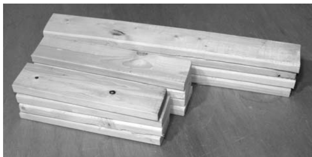
Figure 11-6 1 × 2s used to form the rest of the cage frame
