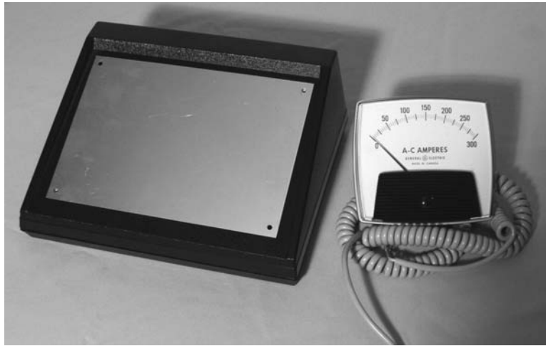
Figure 7-26 A large analog meter and enclosure
