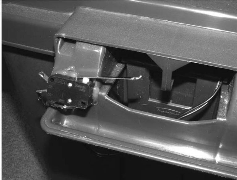
Figure 3-32 Trash can-mounted microswitch
