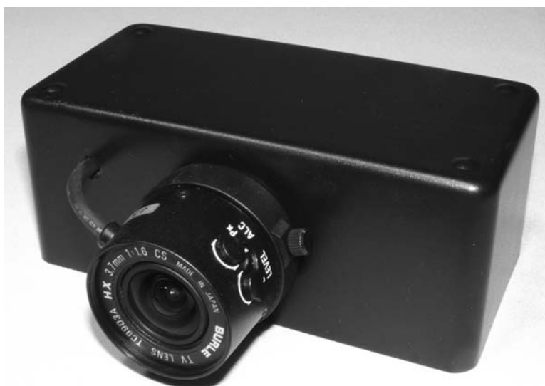
Figure 8-19 Mounting the lens to the enclosure
