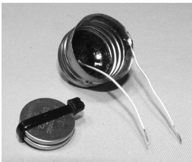
Figure 8-5 Wires soldered to the bulb base
