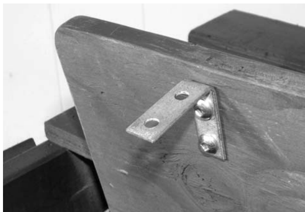
Figure 11-12 A launch-pad locking system made from a shelf bracket
