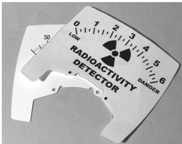
Figure 7-28 Printing out the new meter panel
