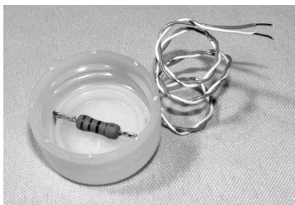
Figure 2-17 The heating resistor installed
