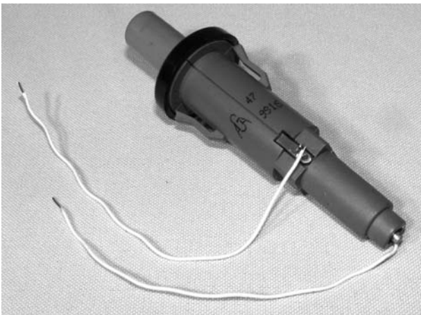
Figure 7-2 Connecting wires to the two terminals
