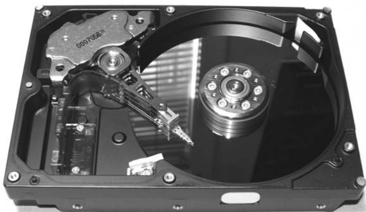
Figure 4-22 Inside a typical hard disk drive
