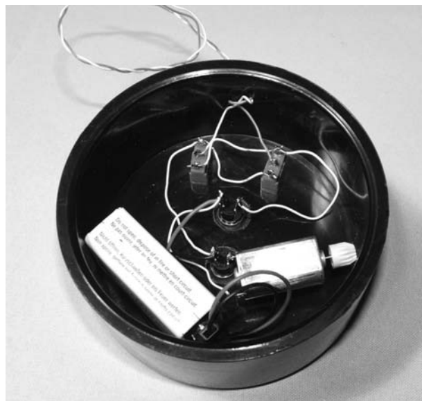
Figure 8-16 Switches and noise motor inside a PVC cap
