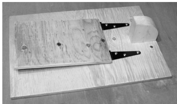
Figure 11-2 Fastening the hinged launch pad to the launch base
