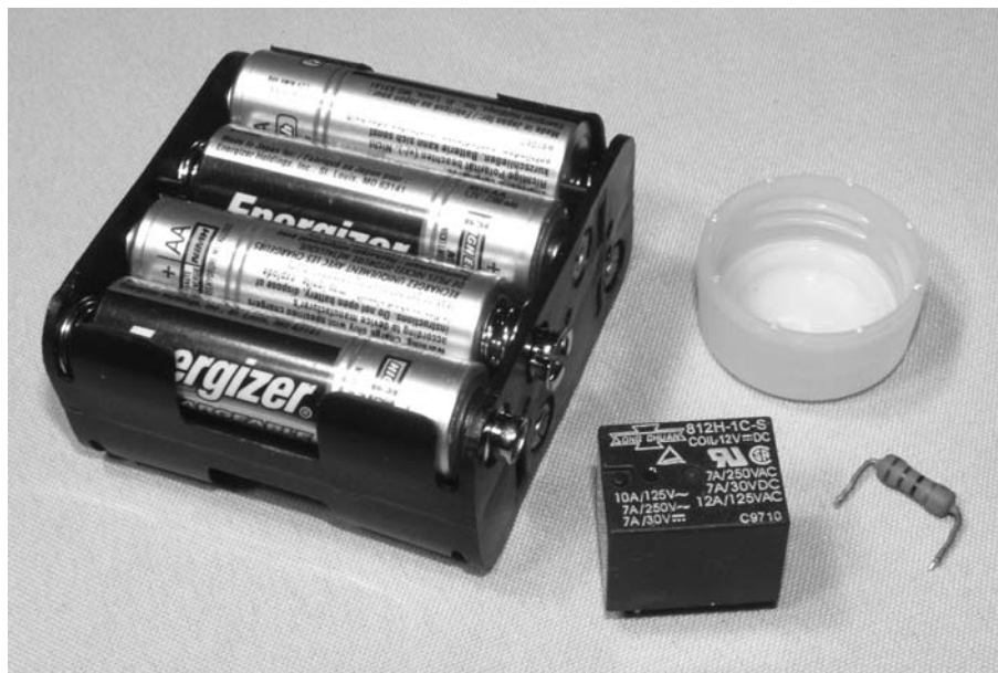
Figure 2-16 Battery pack, resistor and relay
