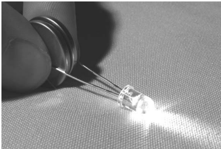
Figure 8-2 Test the white LED with your batteries
