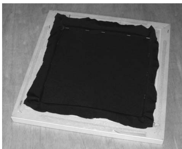
Figure 10-15 Securing the material over the clear glass front
