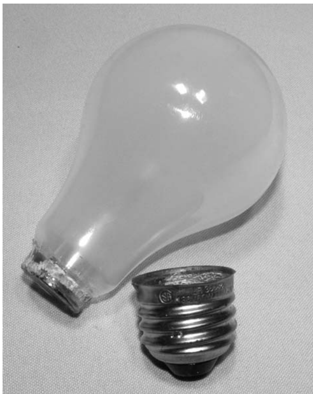
Figure 8-4 Base removed from the bulb
