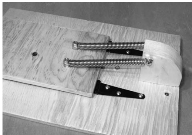
Figure 11-5 Launch springs in the loaded position
