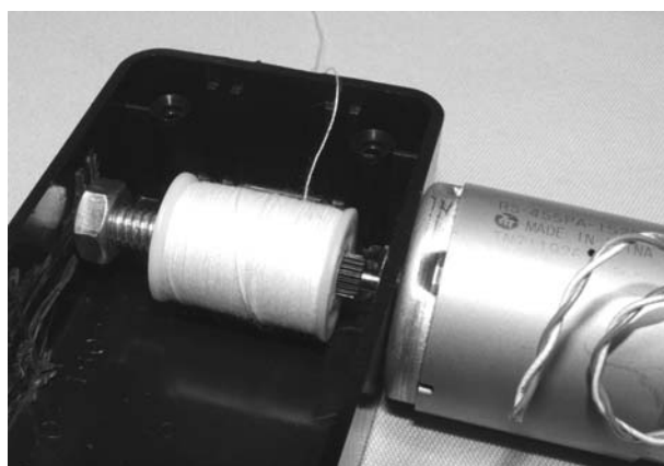
Figure 3-17 Towing mechanics completed
