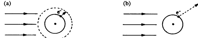
Fig. 2.8. (a) Photoabsorption out of a monochromatic beam of photons: An electron is elevated from a low-lying bound state to a higher-lying bound state. (b) Photoionization: A bound electron is excited into a continuum state
