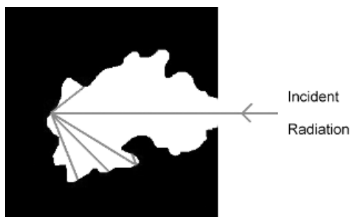
Figure 1.4.1 Cavity radiator absorbing incident radiation.
