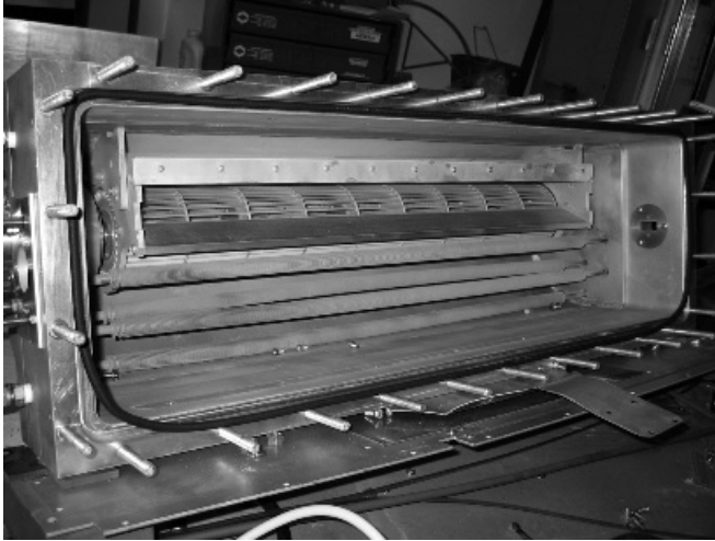
Figure 10.10.5 Excimer laser heat exchanger and fan.
