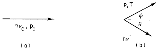
FIGURE 15.4. Momentum relationships in Compton scattering. (a) Before. (b) After. The photon emerges at angle \theta , the electron at angle \phi .
