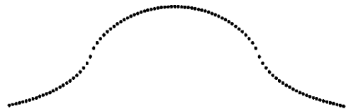
FIGURE 12.23. Reconstruction by simple back projection without convolution. The object is the same as in Fig. 12.22.
