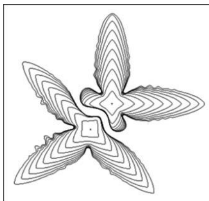
FIGURE 7-6 Contour lines of the interfacial position at \phi = 0.5 for two neighboring Ni-Cu dendrites at different time steps.
