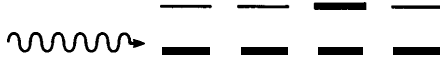
Fig. 7.5. Functioning of a saturable absorber. The wave coming from the left-hand side hits atoms each with two levels (symbolized by horizontal lines) and excites some of them.
