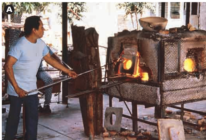
Figure 12.1 (A) When the temperature of a kiln surpasses 1000 K, the radiation is independent of the nature of the material in the kiln and depends only on the temperature. (B) A tiny hole in a very hot cavity “samples” the radiation that is being emitted and absorbed by the walls inside.
