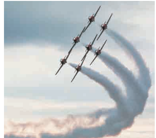
Figure 2.10 When an airplane follows a curved path, it must tilt or bank to generate a centripetal force.
