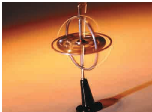
Figure 4.10 When a spinning object begins to fall, its angular momentum resists the direction of the fall.
