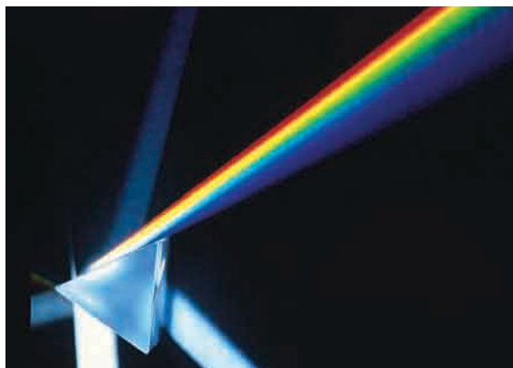
Figure 9.2 Using a refracting prism, white light can be separated into a spectrum of colour.
