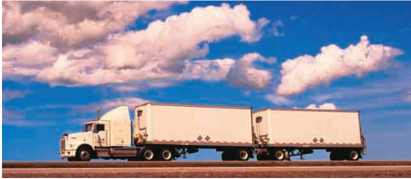
Figure 1.7 This truck and its two trailers move as one unit. The velocity and acceleration of each of the three sections are the same. However, each section is experiencing a different net force.
