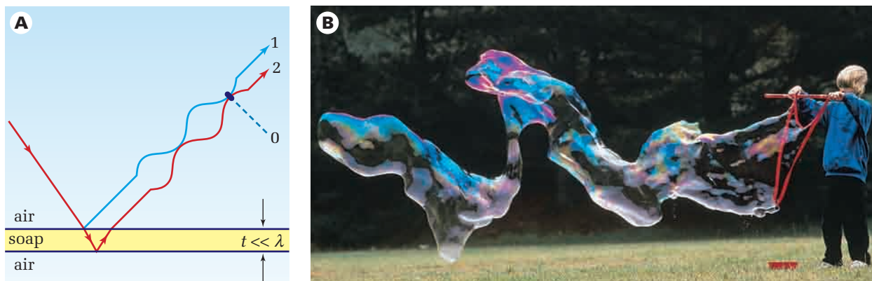
Figure 9.24 (A) Phase inversion causes destructive interference in very thin film when the film thickness, t , is much less than the wavelength of light, \lambda . (B) A soap bubble varies slightly in thickness, causing the destructive interference of varying colours.
