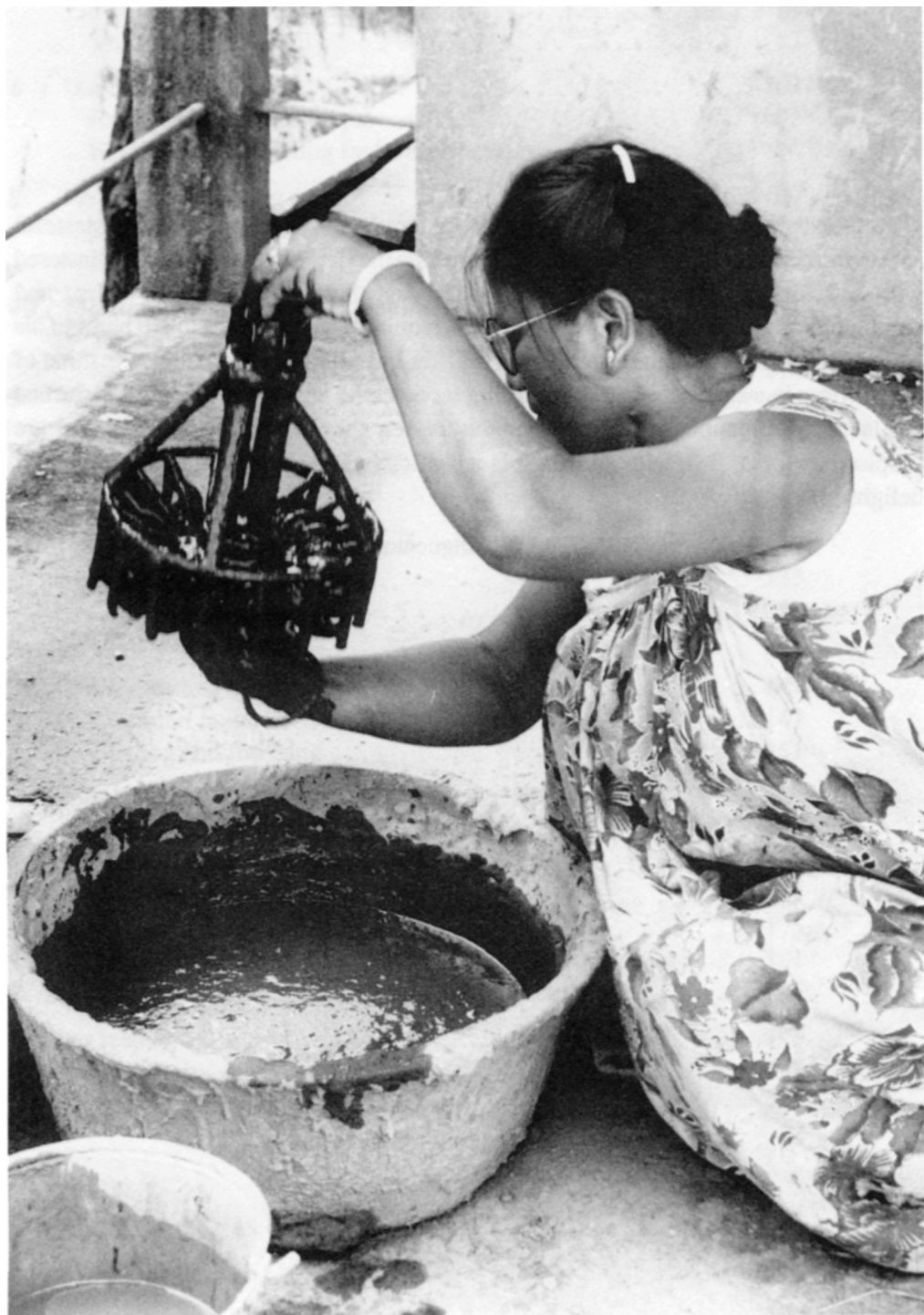
Traditional Newar method of lost-wax casting using a clay-dung slurry investment
