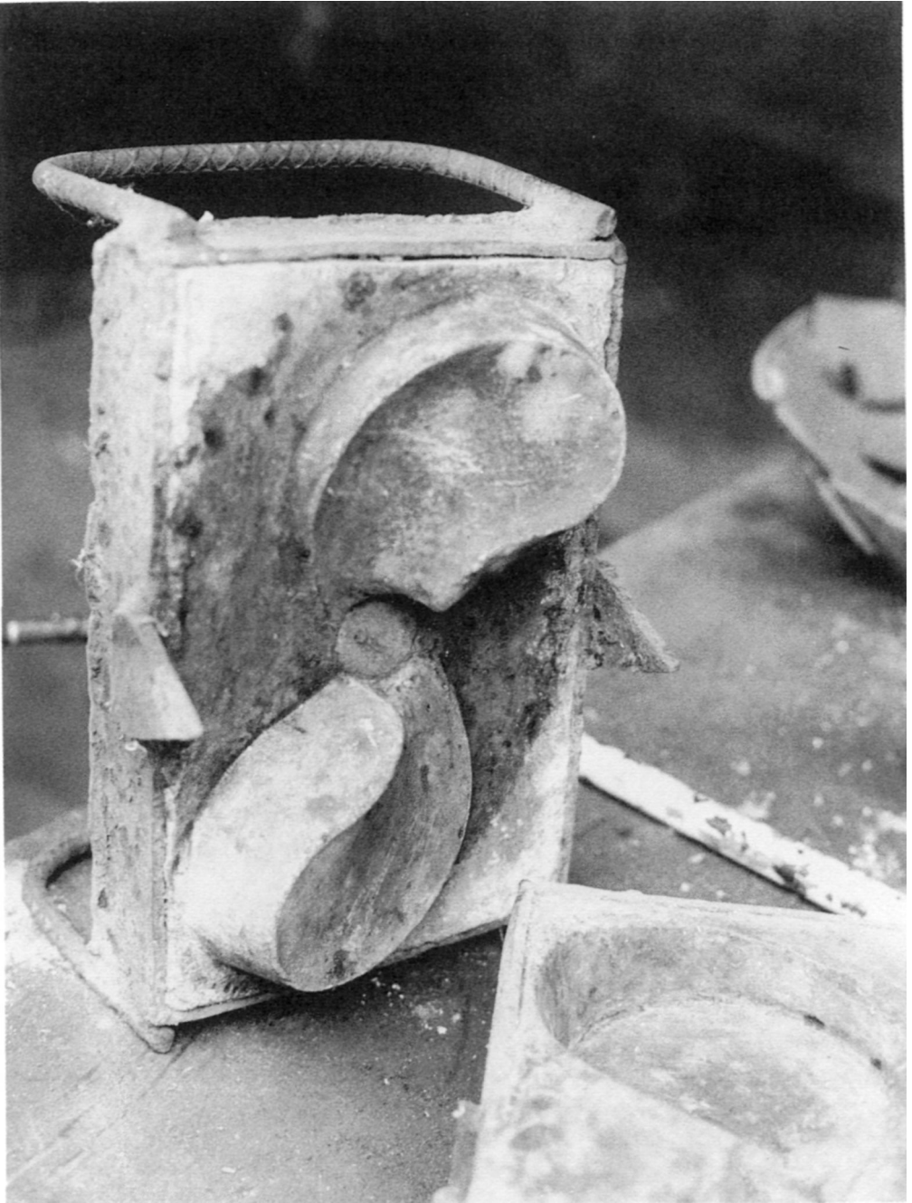
Aluminium die for casting propellers for small river boats in Peru
