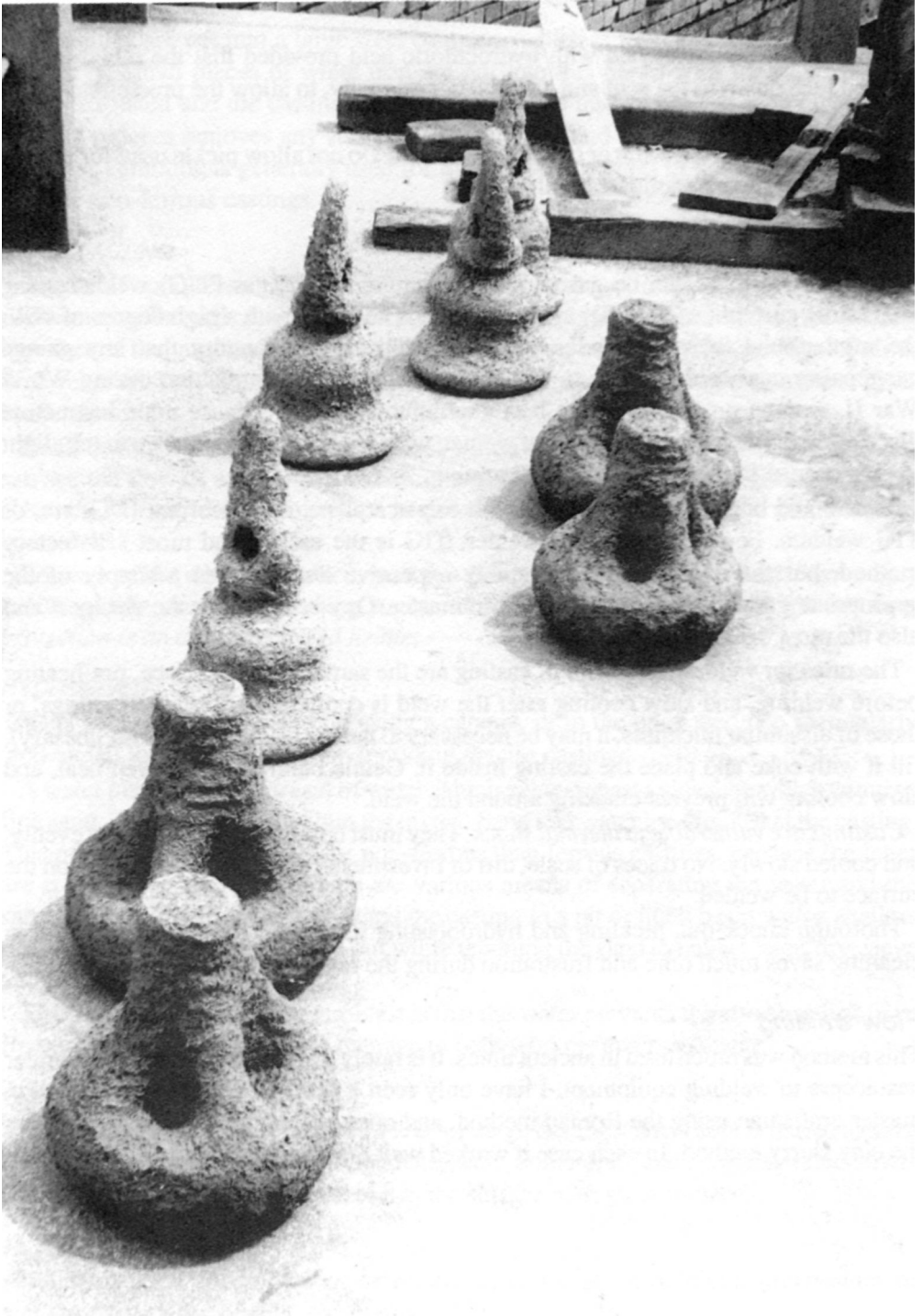
Traditional Nepalese bells (background) and Pelton turbine wheels drying in the sun after first, second and final coats of investment using the Newar method
