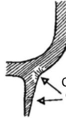
Figure 131. Contraction necessitates the redesign of runner and feeding system
