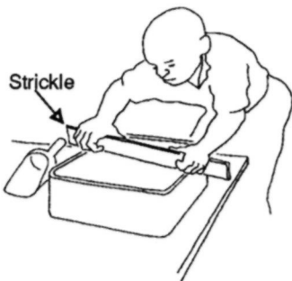
Figure 32. Smooth the surface with the strickle and remove surplus sand
