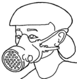
Figure 139. Acid vapour, solvents and many other chemical fumes can damage the lungs: when degreasing, patinating, or using concentrated acid, protect lungs against fumes
