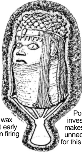
Figure 69. Completed clay slurry mould with wax runners and cup attached
