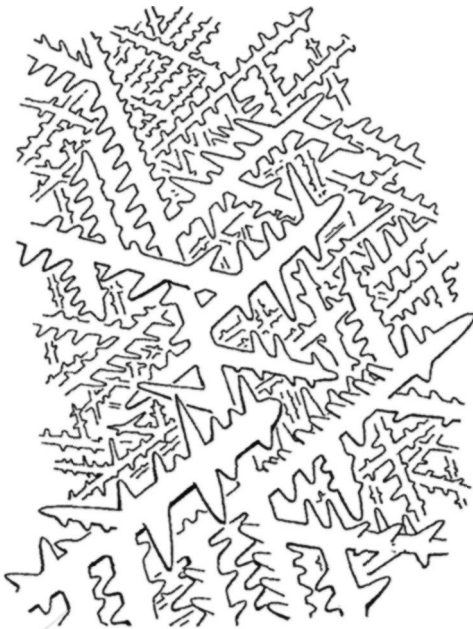
Figure 94. Formation of dendrites as alloy 'freezes'
