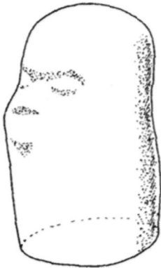
Figure 66. Clay slurry technique: the core is formed from a mixture of clay, straw and horse dung
