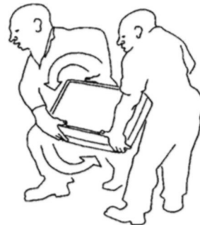
Figure 33. Turn the flask (cope and drag) when it has been filled with sand and rammed tight
