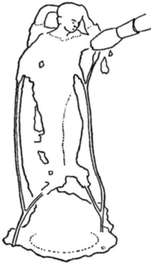
Figure 53. The first coat of the investment is painted onto the wax: take care to remove all air bubbles
