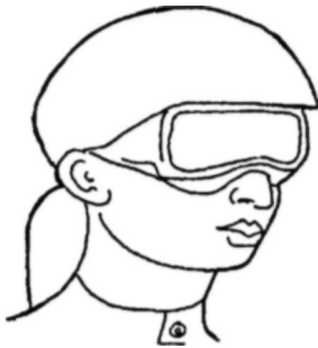
Figure 141. When pickling castings, protect eyes, hands and skin against weak acid
