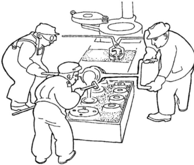
Figure 90. An Italian foundry in the 1960s: the boss takes charge of pouring; his assistant wears goggles - the exception rather than the rule as bronze casters disliked protective clothing, saying that it made the foundry workers clumsy, but protective clothing is now compulsory throughout the EU.
