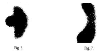
Several grains of radio-active matter are put on a photographic plate enveloped in black paper and placed horizontally between the poles of a magnet; on developing the plate after a few moments' exposure, it will be seen that beside the mark indicating the position of the active source a strong impression has been produced due to the radiation reflected by the field and collected on the plate, on one side only.
