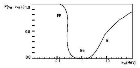
**FIGURE 11.** Energy dependence needed for  $P(\nu_e \rightarrow \nu_e; L)$  to fit the solar neutrino data.[54]
