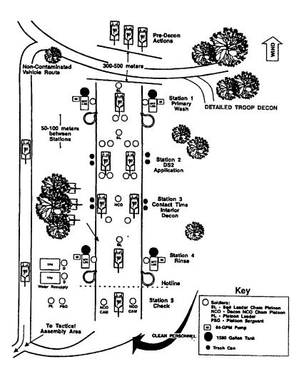
Figure 3-8. An Alternate DED layout for an M17 LDS-equipped unit.
