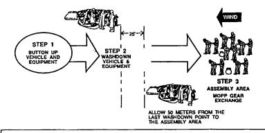
Unsupported one-lane washdown with one lightweight decontaminating system (shown below) and with two lightweight decontaminating systems (above)
