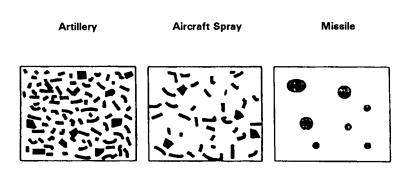
Figure 1-2. Moderate liquid contamination on M9 paper (1 gram/square meter).
