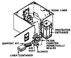
Figure 2-8. Simplified collective-protection equipment.
