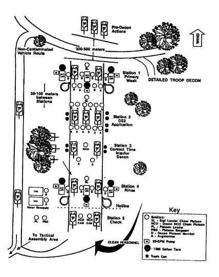
Figure 3-7. Optimum DED layout for an M17 LDS-equipped unit.
