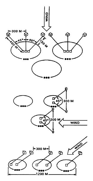
Figure 3-1. Fixed emplacement of M8A1 alarms.
