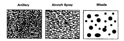
Figure 1-1. Heavy liquid contamination on M9 paper.
