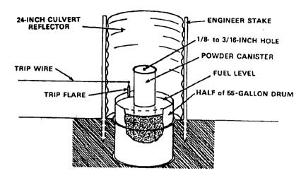
Figure 7-6. Cutaway showing composition of a Husch flare.
