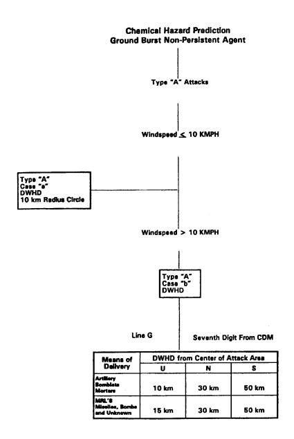
Figure 2-2. Flow chart, type A attack.
