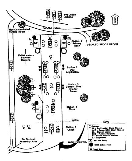
Figure 3-6. An Alternate DED layout for an M12A1 PDDA-equipped unit.
