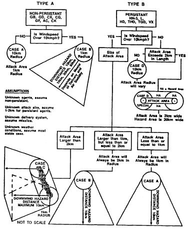
Figure 2-1. Flow chart. Chemical Hazard Prediction
