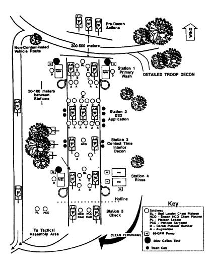
Figure 3-5. M12A1 PDDA-equipped unit-optimum DED layout.
