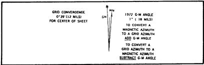
Figure D-1. Typical declination diagram.
