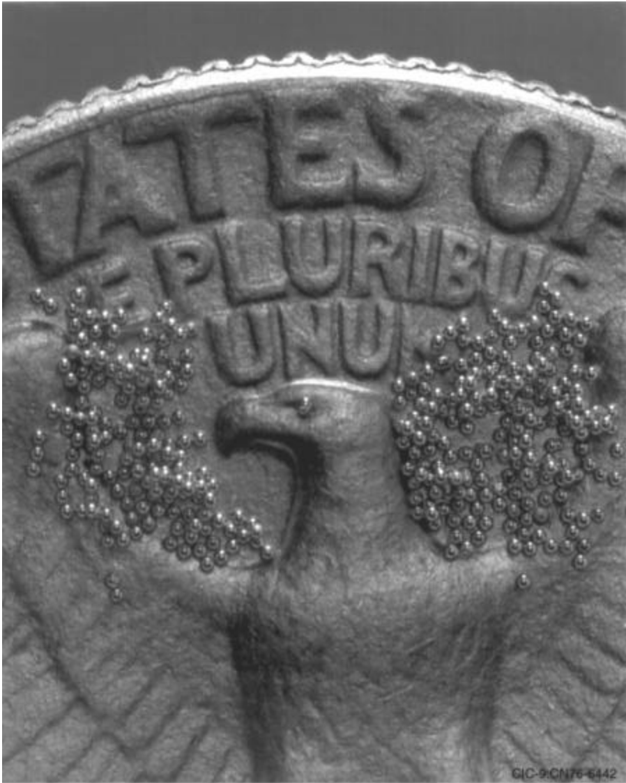
FIG. 14.5 Gold microshells containing high pressure D-T gas for use in laser fusion (Courtesy Los Alamos National Laboratory, No. CN 76-6442).
