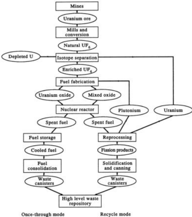
FIG. 22.1 Nuclear fuel cycles. The once-through shown on the left is used in the U.S.; the recycle shown on the right is used in other countries.
