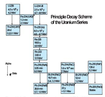
Figure 25-5. Uranium-238 decay series. (From NCRP, 1987.)
