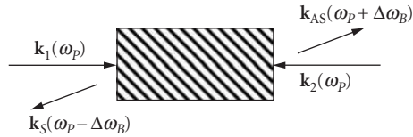
FIGURE 21 k vector diagram for Brillouin-enhanced four-wave mixing.
