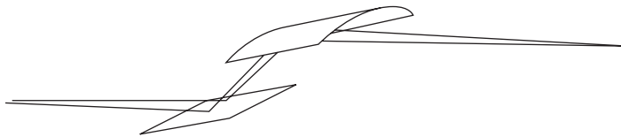
FIGURE 6 The usual arrangement of a sagittally focussing monochromator, with the bent element as the second one of a two-crystal monochromator.
