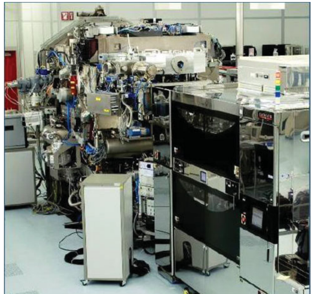
FIGURE 34.2 ASML alpha demo tool during installation. The whole system is under vacuum, and a plasma source is used to generate the EUV radiation (not shown).
