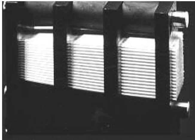
FIGURE 3 Multifiber collimating lens constructed from over a thousand individual polycapillary fibers strung through a metal grid. The lens is 10 cm long with an output of 20 \times 20 mm. The fibers are parallel at the output end (shown) and at the input end point to a common focal spot.
