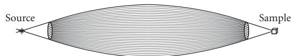
FIGURE 4 Sketch of the interior channels of a monolithic polycapillary optic. Monolithic optics can be focusing, as shown, or collimating, as in Fig. 3. (Sketch from Ref. 14.)
