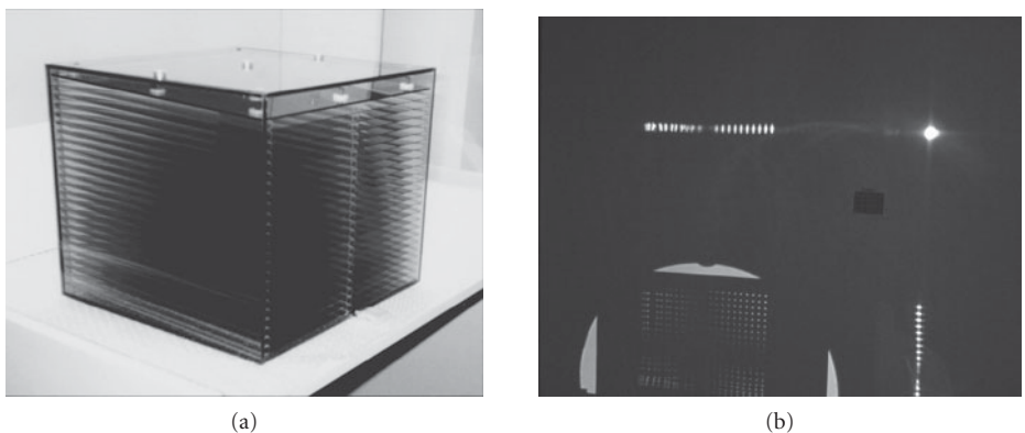
FIGURE 3 Kirkpatrick-Baez test Au-coated glass foils system (a) and VIS focal image (see also color insert) (b) studied for XEUS project. (Courtesy of Reflex.)
