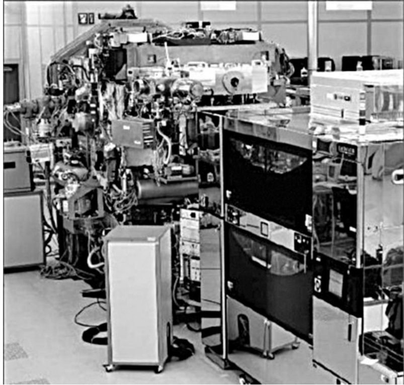
FIGURE 2 ASML alpha demo tool during installation. The whole system is under vacuum, and a plasma source is used to generate the EUV radiation (not shown). 8 (See also color insert.)
