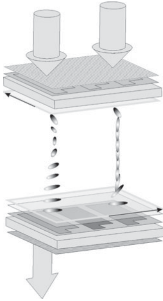
FIGURE 21 The basic operation principles of the TN cell.
