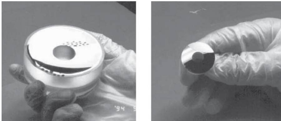
FIGURE 4 Mirrors forming a Schwarzschild objective during assembly.
