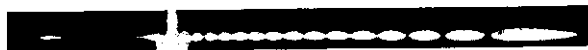
Fig. 17.12 Observed spectral broadening in a mixture of \text{CS}_2 and benzene with a multimode Q -switched ruby laser pulse. [After T. K. Gustafson, J. P. E. Taran, H. A. Haus, J. R. Lifshitz, and P. L. Kelley, Phys. Rev. 177 , 306 (1969).]
