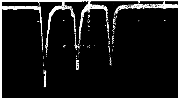
Fig. 21.8 Oscilloscope trace (100 nsec/division) showing the photon echo from a ruby sample at 4.2 K. The echo appears as the third pulse following the two exciting pulses from a ruby laser. (After Ref. 12.)
