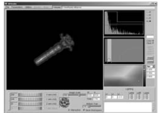
Figure 7.23 A transfer function editor with an HSV color palette and a mapping of densities to various material properties. (See also color insert.)
