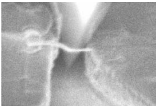
Figure 46.12 A carbon nanotube welded to both sides of the test structure being probed using the AFM.
