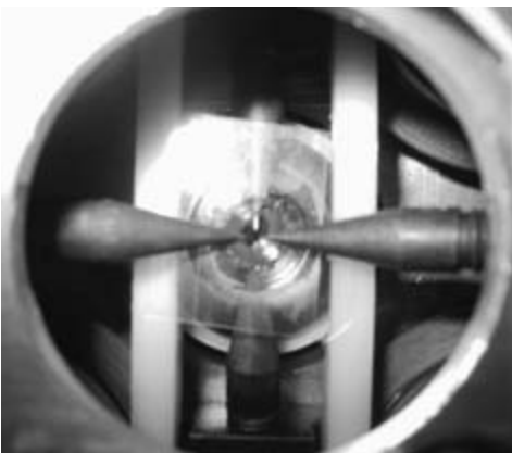
Figure 46.15 Photograph of four magnetic poles in a 3DFM surrounding a specimen mounted between two cover slips. (See also color insert.)
