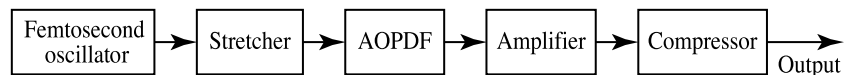
Figure 8.21 Typical configuration for using an acousto-optic programmable dispersive filter in an amplified femtosecond system.
