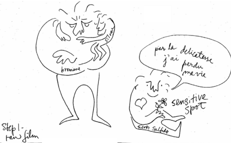
Figure 5.11. Prior to exposure, the photosensitive grain is composed of a silver bromide single crystal with silver sulfide impurities or sensitive spots introduced during manufacture. The bromine atoms are so large that they stay fixed in place, but the silver atoms are smaller and much more mobile. Professor Shelly Errington of the University of California at Santa Cruz drew this original illustration.
