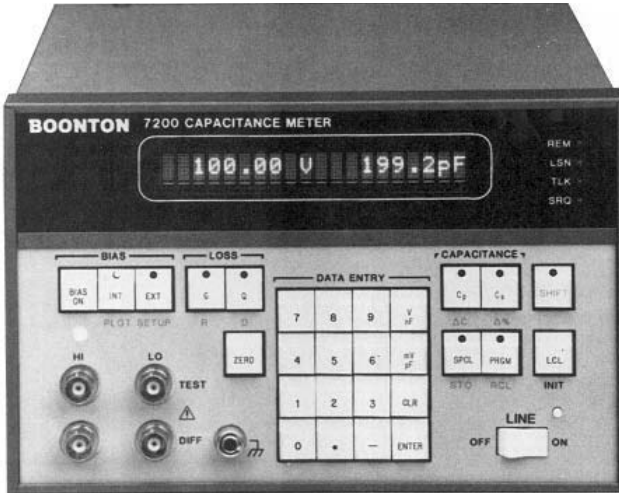
Figure 4.6. The front panel of a capacitance–voltage meter showing a measured value of 199.2 pF at a diode bias of 100 V. This instrument can measure both conductance (charge flow in phase with the voltage) and capacitance (charge flow 90° behind the voltage).
