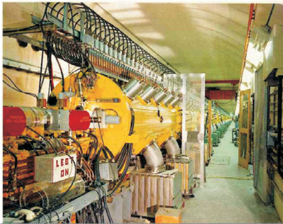
Photo 2: A view of the linac at RHIC. Its purpose is to provide currents of up to 35 milliamperes of protons at energies \approx 200 MeV for injection in a synchrotron for further acceleration. The basic components of the linac include a radiofrequency quadropole pre-injector, and nine accelerator radiofrequency cavities spanning the length of a 150 meters tunnel (shown above.) [Courtesy of Brookhaven National Lab.]
