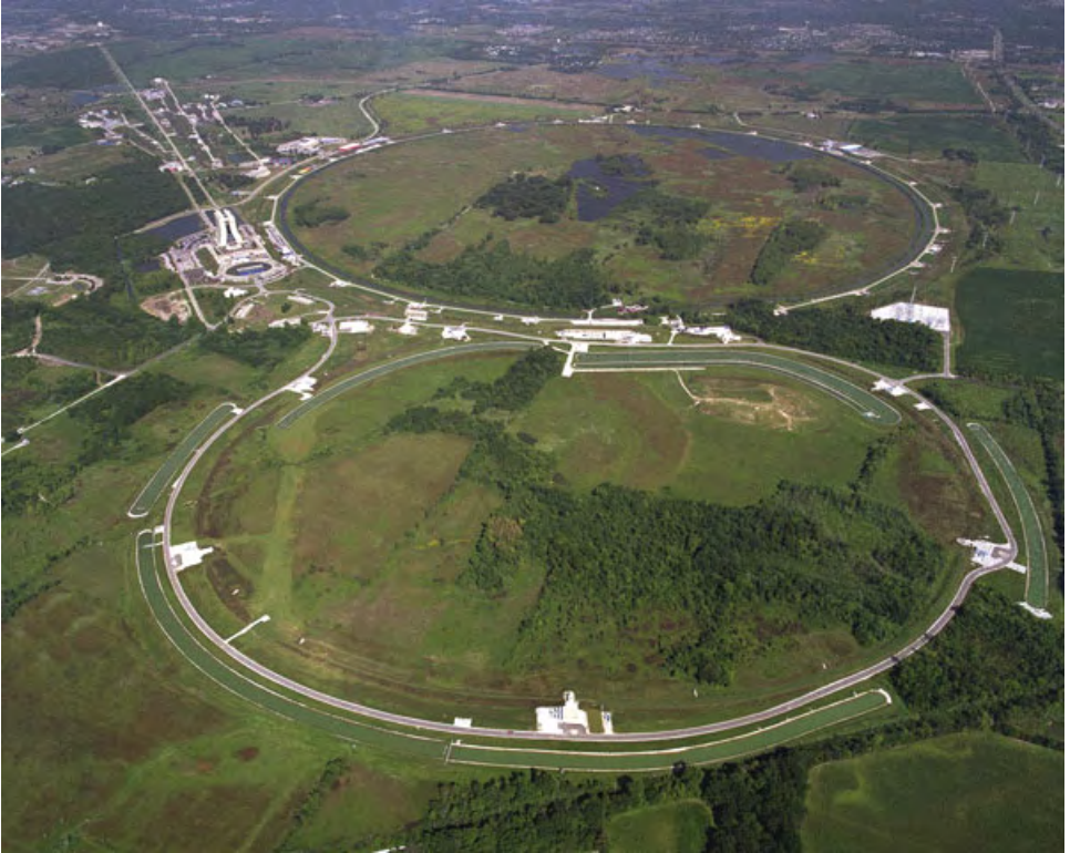
Photo 4: Aerial photograph of Fermi National Accelerator Laboratory (FNAL), at Batavia, Illinois. The beam originates at the top left and is accelerated in the linac (visible as a straight line) to get into the main injector (the bottom ring) where it is brought to 150 GeV. The Tevatron is the top ring, approximately 2 kilometers in diameter, where the beam is accelerated to 1 TeV. (Courtesy Fermi National Accelerator Laboratory.)
