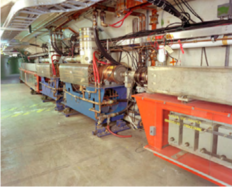
Photo 3: The photographs a-d show the essential parts of the 1 TeV proton synchrotron (Tevatron) at the Fermilab. Protons are accelerated to 750 keV in an electrostatic accelerator (Cockcroft–Walton, photo a); a linear accelerator (photo b) then brings the energy up to 400 MeV and injects the protons into a booster synchrotron. The booster synchrotron (photo c) raises the energy to about 8 GeV and the main ring (lower on photo d) to 150 GeV. The final energy of approximately 1 TeV is achieved in the Tevatron ring. [Courtesy Fermilab.]
