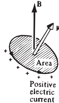
Figure 5.3: A current loop gives rise to a magnetic moment \mu . The direction of the magnetic moment is perpendicular to the plane bounded by the current.
