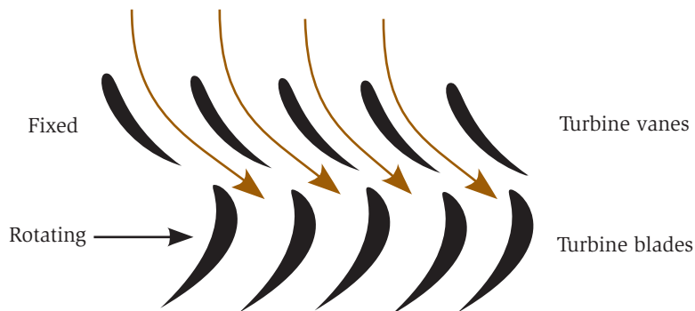
Fig. 5.17. The turbine with its vanes and blades.
