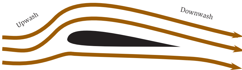
Fig. 2.3. The airflow around a real airfoil looks like this.
