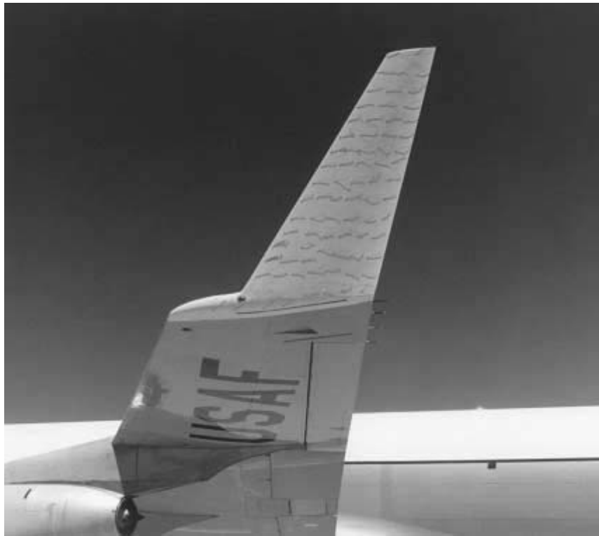
Fig. 3.18. A winglet on a K-C135A. (Photo courtesy of NASA.)
