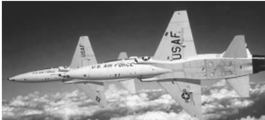
Fig. 6.13. Two T-38 Talons with fuselage “waist.” (Photo courtesy of the U.S. Air Force.)
