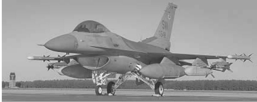
Fig. 2.23. Armament goes on the bottom of the wing of an F-16. (Photo courtesy of the U.S. Air Force.)
