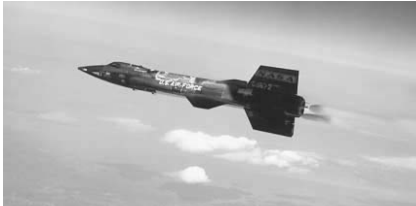
Fig. 6.16. The rocket-propelled X-15. (Photo courtesy of NASA and the U.S. Air Force.)
