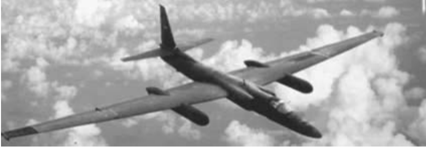
Fig. 3.5. A U-2 with a high aspect ratio wing. (Photo courtesy of the U.S. Air Force.)
