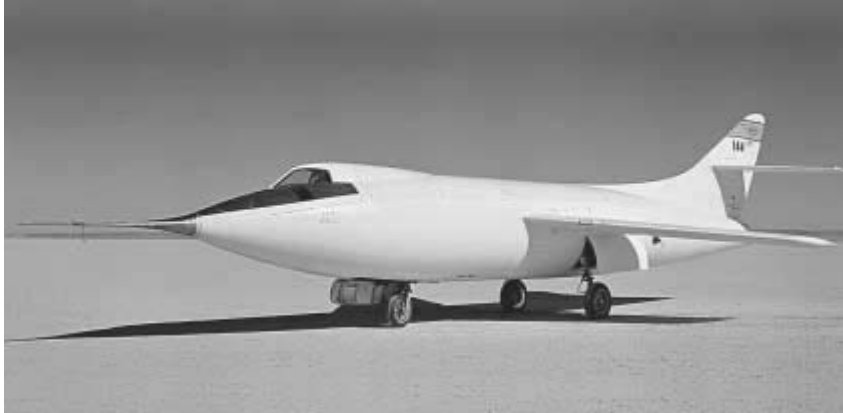
Fig. 8.22. Airspeed calibration probe on D-558-II. (Photo courtesy of NASA.)
