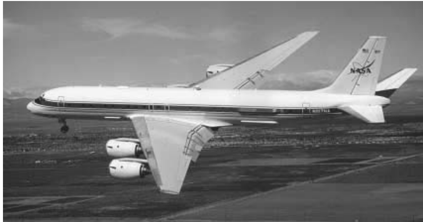
Fig. 3.9. The DC-8 illustrating wing taper. (Photo courtesy of NASA.)
