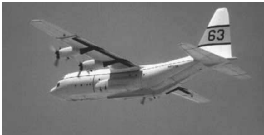
Fig. 3.16. The C-130 Hercules demonstrating fuselage upsweep. (Photo courtesy of Paul Burke.)
