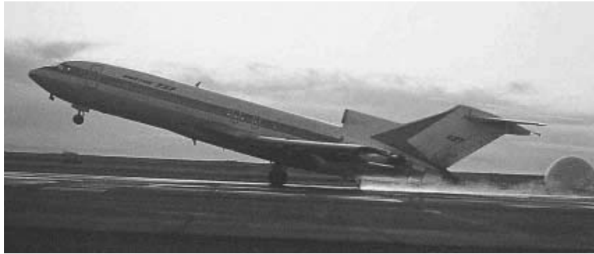
Fig. 8.24. VMU test with a tail skid on the airplane to prevent damage. (Used with the permission of the Boeing Management Company.)
