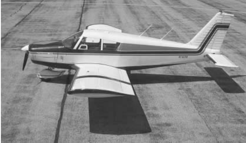
Fig. 3.11. Piper Cherokee 140 with a “Hershey Bar” wing. (Photo courtesy of Albert Dyer.)
