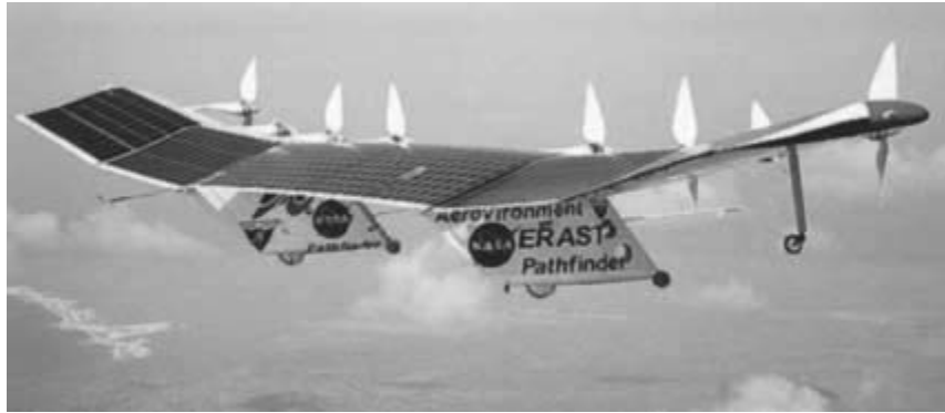
Fig. 7.9. Pathfinder, a maximum endurance, solar-powered airplane. (Photo courtesy of NASA.)
