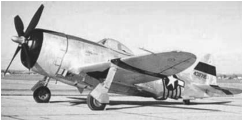
Fig. 3.12. The Republic P-47 with an elliptical wing shape. (Photo courtesy of the U.S. Air Force Museum.)
