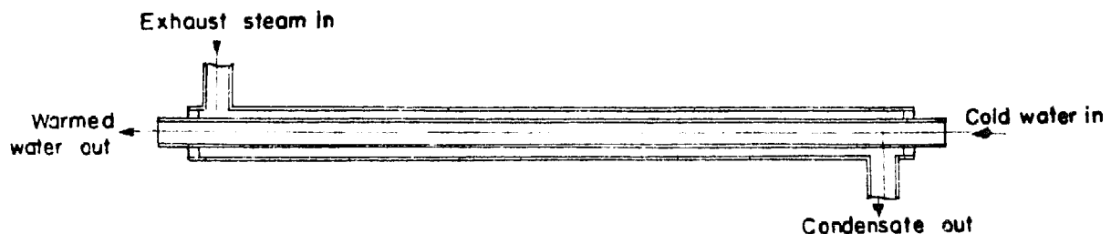
Fig. 8-6: Contra flow principle feedheater
