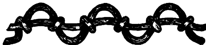
Cleaveland's Undulating Visible Wire Fencing 40 Two-strand undulating ornamental wire. Outer strand loops and wraps around central undulating strand. Patented [475719] May 24, 1892, by John B. Cleaveland of Indianapolis, Ind.
