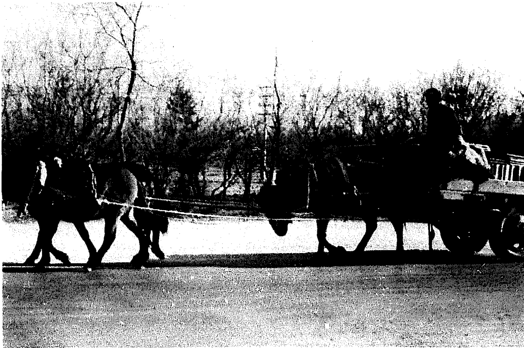
Figure 2.23 A single animal can support the load while others pull on traces: China.
