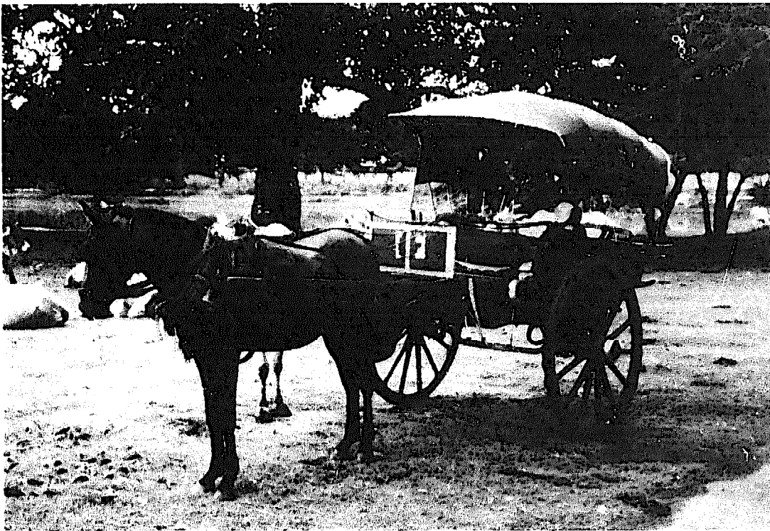
Figure 2.3 Two-wheeled passenger cart. Horse is hitched to cart with collar harness and saddle: Burma.
