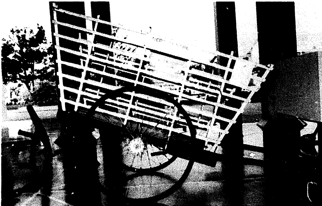
Figure 2.37 Tension-spoked steel wheel: Sri Lanka. Source: Economic and Social Commission for Asia and the Pacific
