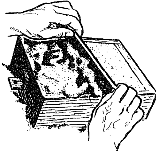
Fig. 59. Strickling away the surplus sand.
