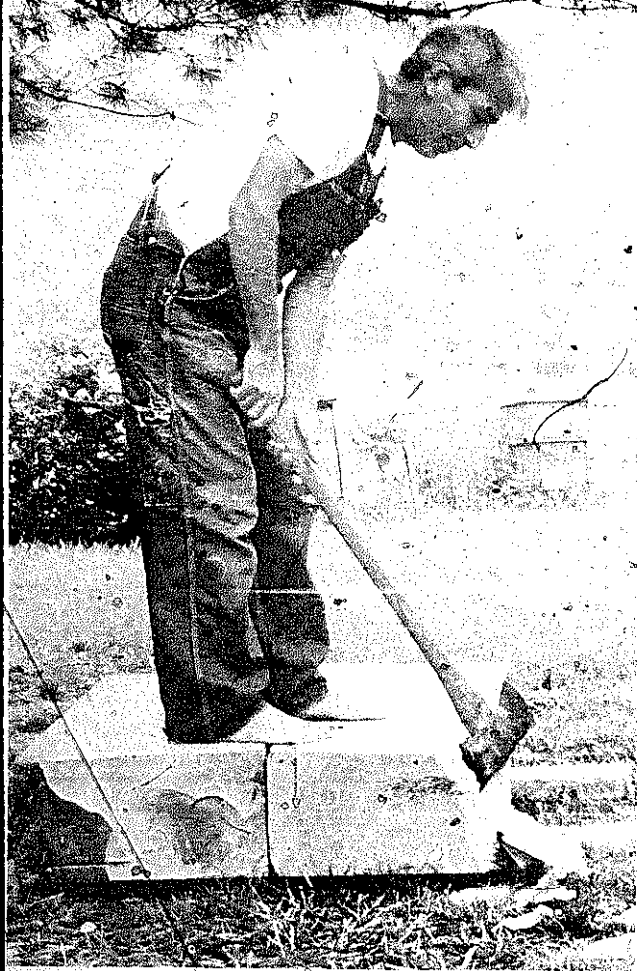
PLATE 137 With an axe, he hews the wheel out round.
