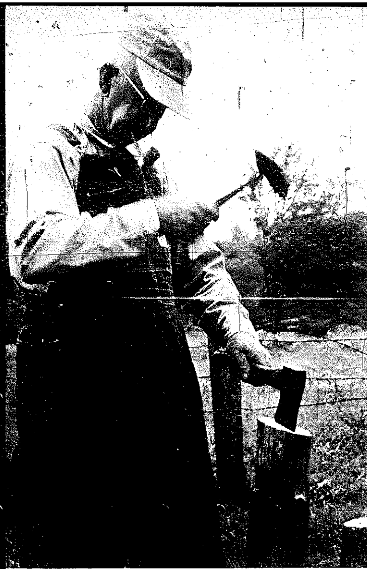
PLATES 320-322. Mr. Dickerson notches the ends of the three legs to fit the battling bench, and then nails them into place. The bench has three legs so that it will set steady, even on rough ground.
