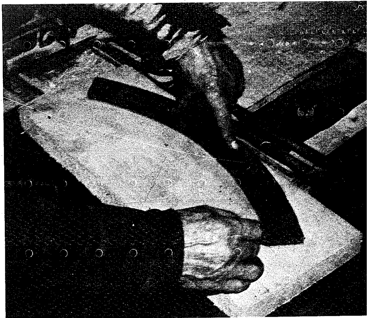
PLATES 90-93 A pattern is made for the wooden rim of the wheel (Plate 90), and the six felloes marked out on inch-and-a-half thick oak stock (Plate 91). Traditionally, these were cut out with a felloe saw (Plates 92-93 on p. 124).
