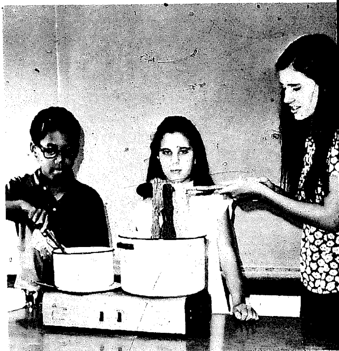
Skeins being lifted from pot to show effect of different mordants. Mordants (chemicals) control final dye colors.
