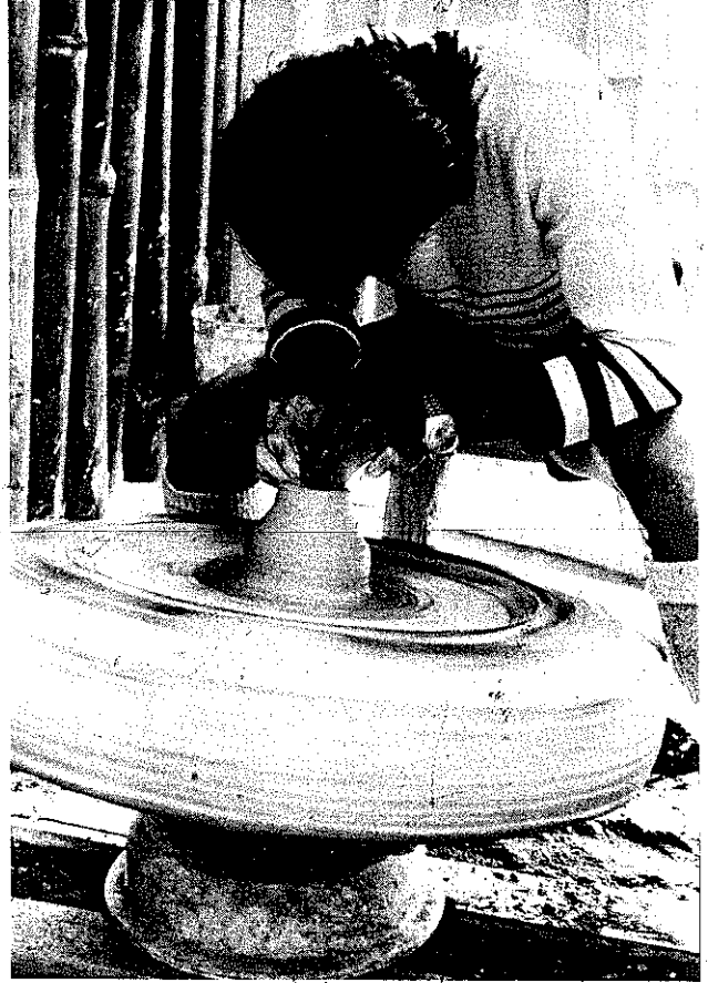
POTTER'S WHEEL. Make it spin fast by turning it with a pointed stick in a small hole in the concrete. The wheel is heavy enough that with practice you can throw a pot with each spin.
