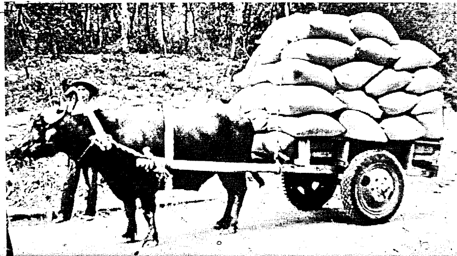
A single-harness bullock-drawn cart in China. The cart is nominally improved with pneumatic tyres, and has a traditional yoke partially but simply modified for animal comfort. The single-harness cart is carrying about a tonne of bran or husk. Courtesy: W. Ross Cockrill; FAO; op. cit.
