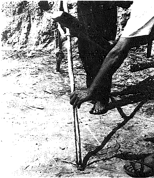
1. Stand the "A" Frame upright. Using the stakes, mark the points where the legs of the "A" Frame touch the ground.
